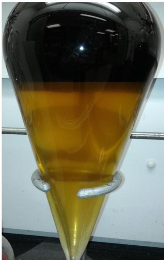
Figure 39. Phase separation during the lignin recovery process.
