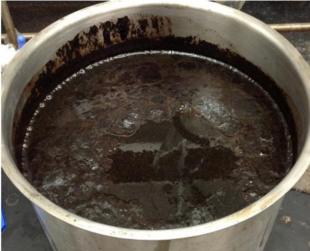
Figure 36. Collection vessel containing black liquor from a -2 solvent run.
