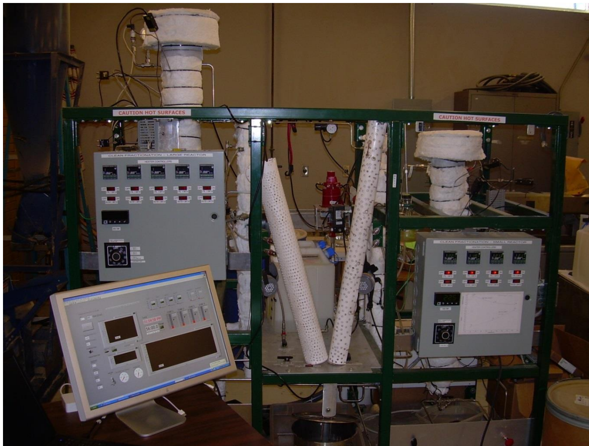
Figure 15. Organosolv fractionation reactor at the CRC, University of Tennessee.
