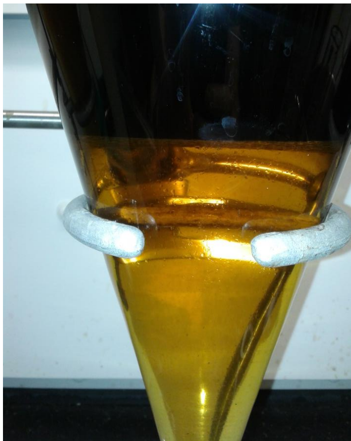
Figure 17. Phase separation between organic (upper) and aqueous (lower) phase.
