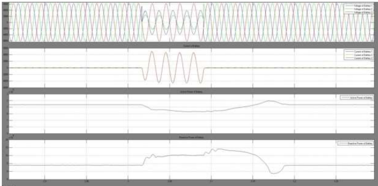
Figure 6.4.V, I, P and Q of Battery.
