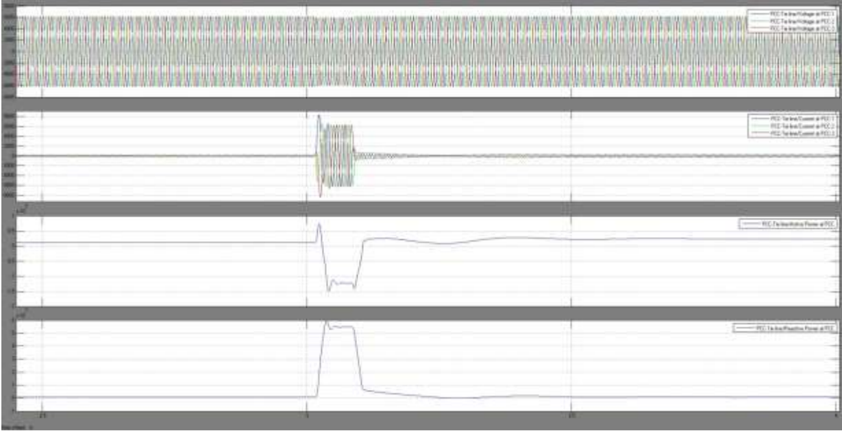
Figure 6.9. V, I, P and Q at PCC
