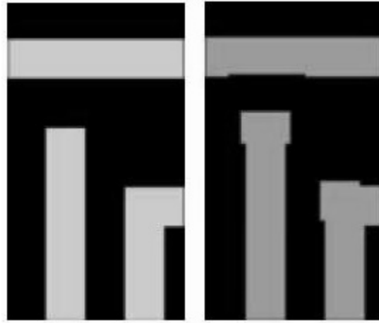
Figure 3.2: Proximity correction based on shape modulation [37]
