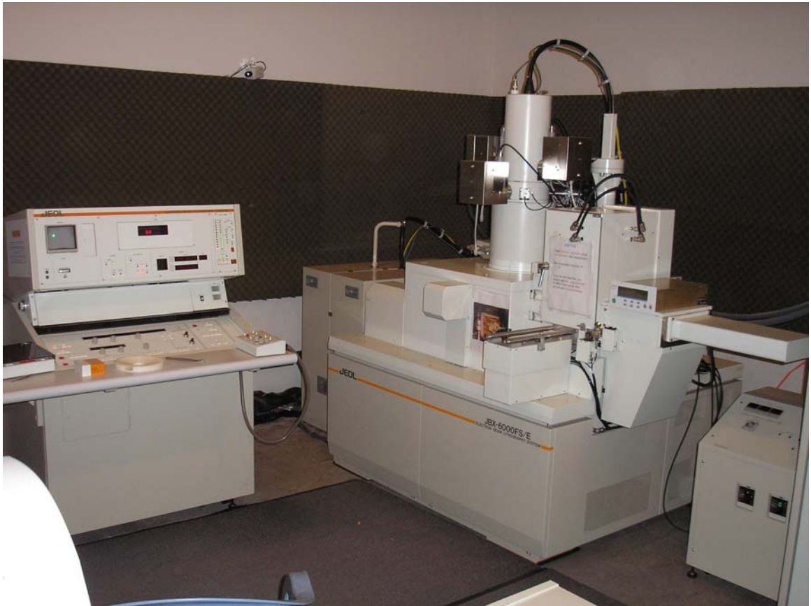
Figure 2.8: Electron Beam Lithography tool - JBX 6000 FS/E (JEOL)
