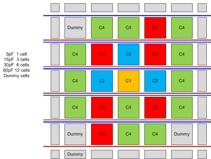
Figure 16: Block diagram illustrating the common centroid technique utilized to layout the capacitors of the OTA- C^4 filter cell with unit capacitors.
