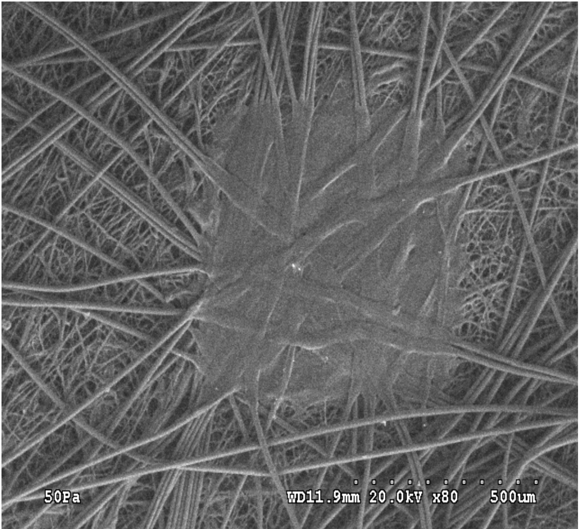
Figure 13. SEM image of SM sample (300°F, 270 PLI, 25%PP/75%PE)
