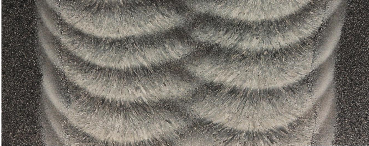
Figure 25. Weld cross-section of narrow gap SAW in the as welded condition, Noren’s reagent, 6X [71].
