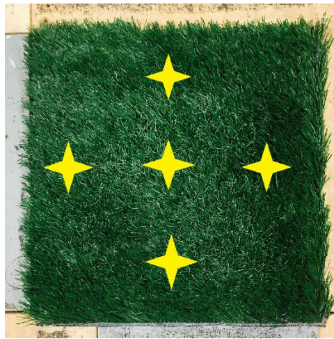
Figure 2. Locations for mechanical test.
