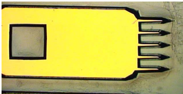
Figure 5.4: Microscope image of needle after three hours of KOH etching showing a modification of the needle tip shapes with respect to the original mask, owing to anisotropic etch characteristics of KOH
