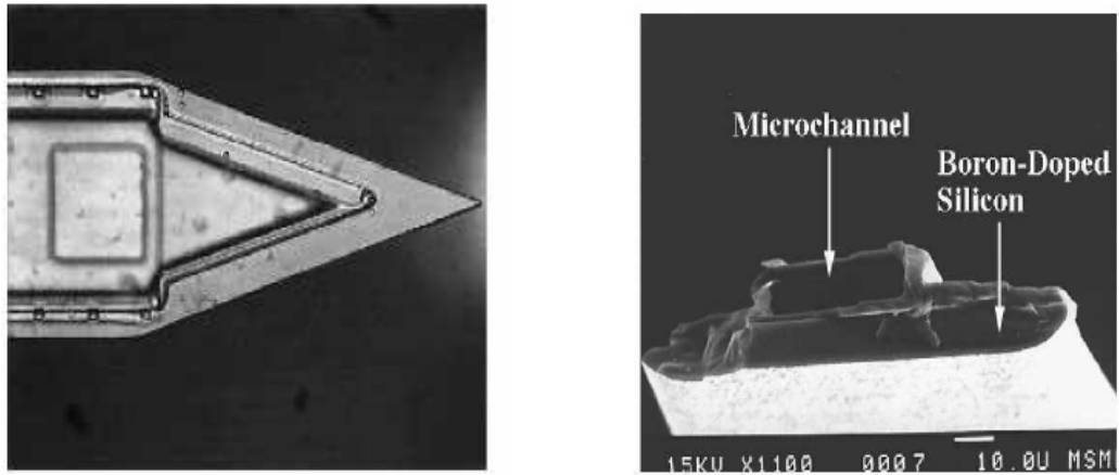
Figure 2.4: [Left] Top view of needle and reservoir; [Right] View of cross-section of microchannel [16]
