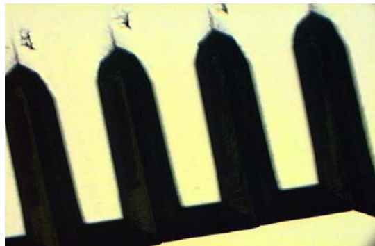
Figure 5.10: Microscope image needles after two hours of KOH etching showing loss of needle shape due to anisotropic etch characteristics of KOH, and needles being etched away well before their release
