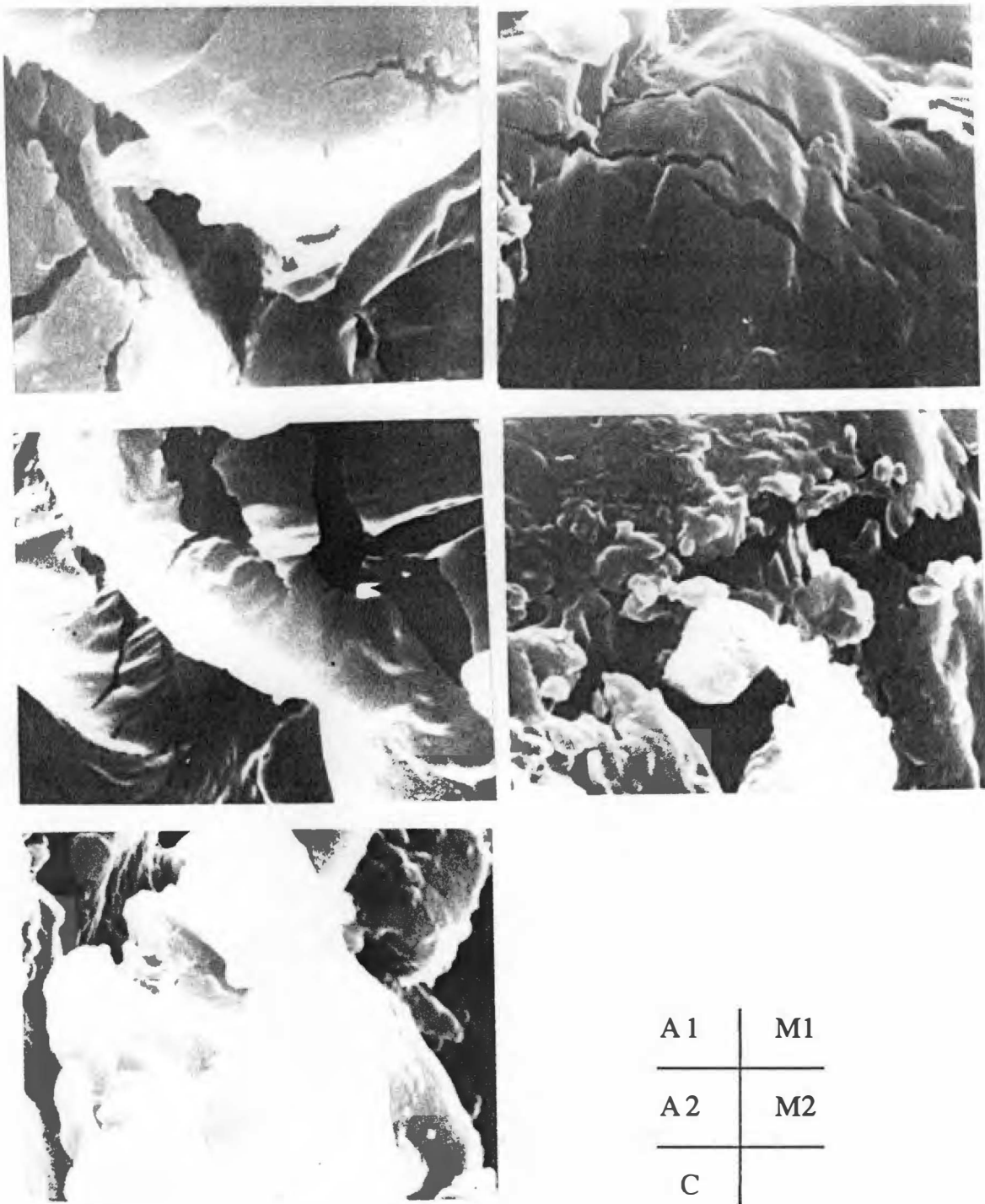
Figure 5—Scanning electron micrograph of apple fiber (X8000). C, control; A1, autoclave 121°C, 15 minutes; A2, autoclave 100°C, 30 minutes; M1, microwave 5 minutes; M2, microwave 10 minutes.
