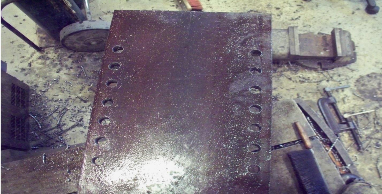
Figure 27. Vertical beams with predrilled holes at 2" spacing.
