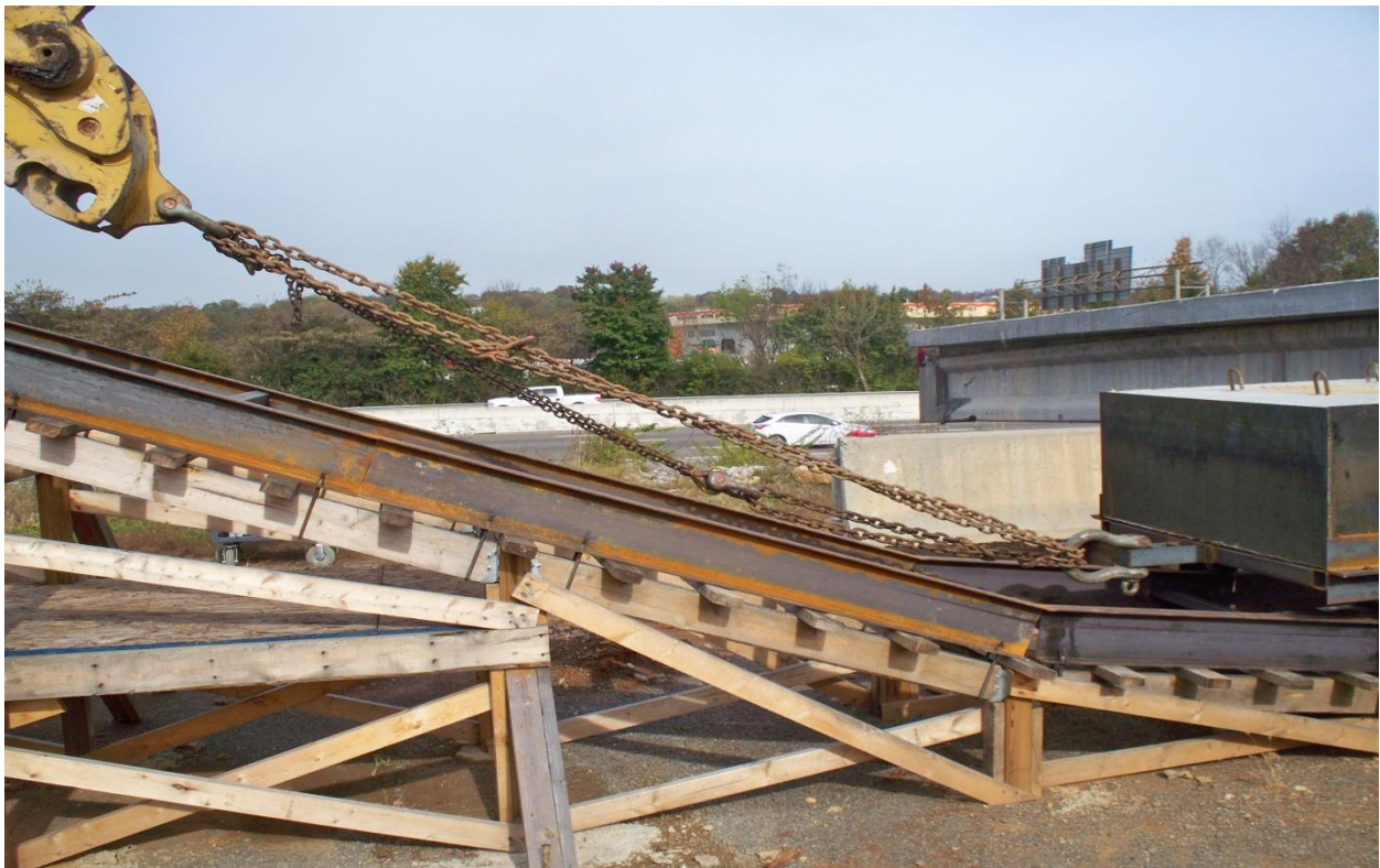
Figure 30. Impact cart hooked up to excavator by shackles and chain.
