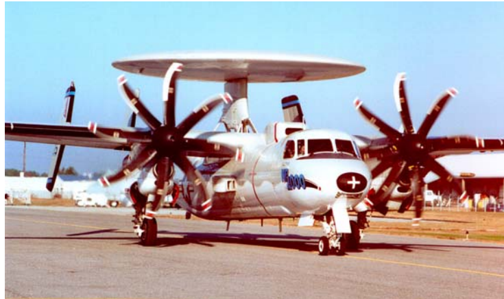
Figure 2. Model NP2000 Propeller Installed on Test Airplane Source: NP2000 ITT Archives, photo by Vernon Pugh.
