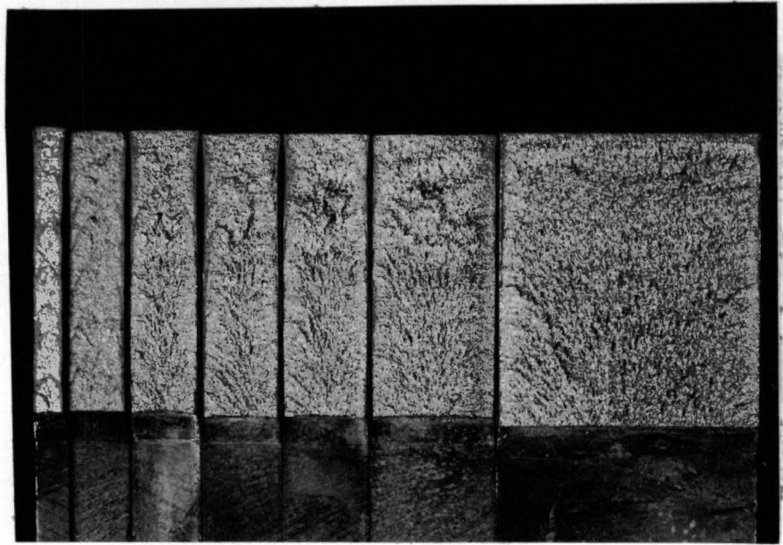
Figure 21. Fracture Surface Appearance as a Function of Specimen Thickness.
