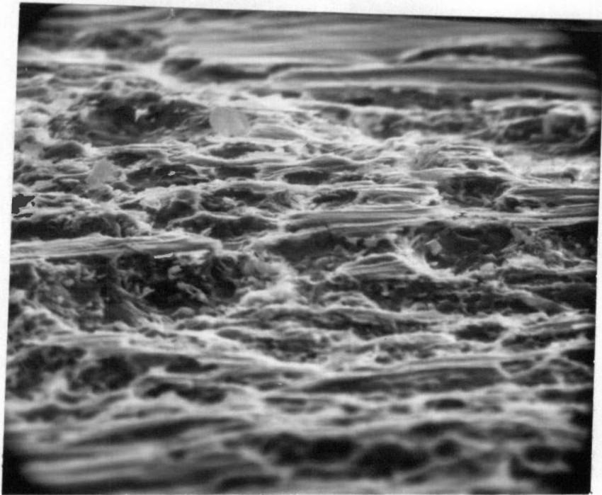
Figure 47. SEM Fractograph of the 0.125 Inch Specimen. Photograph Taken at the Plan View Surface in the Vicinity of the Shear Lip. Mag.: 2000X.
