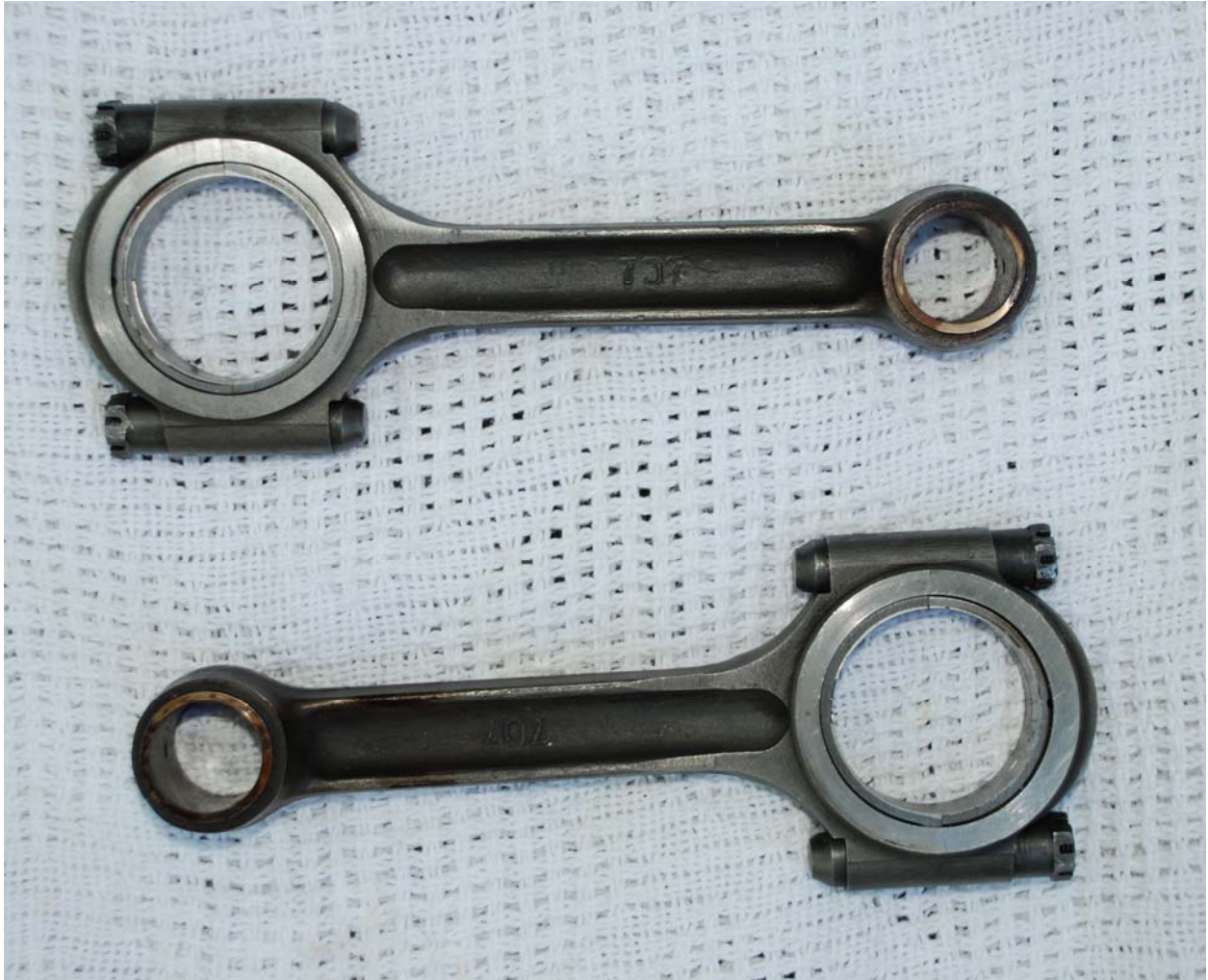
Figure F-5: Forged connecting rod pair with bronze wrist pin bushings, split Babbitt crank pin bearing, and close tolerance clamp bolts/nuts
