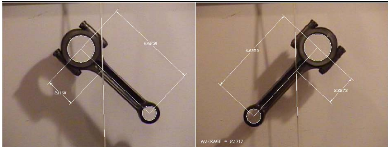
Figure 2-4 Determination of connecting rod CG by suspending from two points
