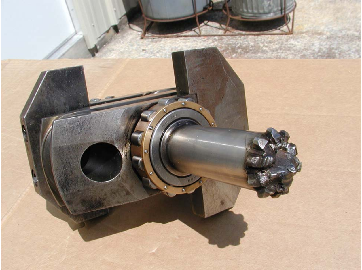
Figure 1-3 E-113 crankshaft failed due to fatigue at root of spines
