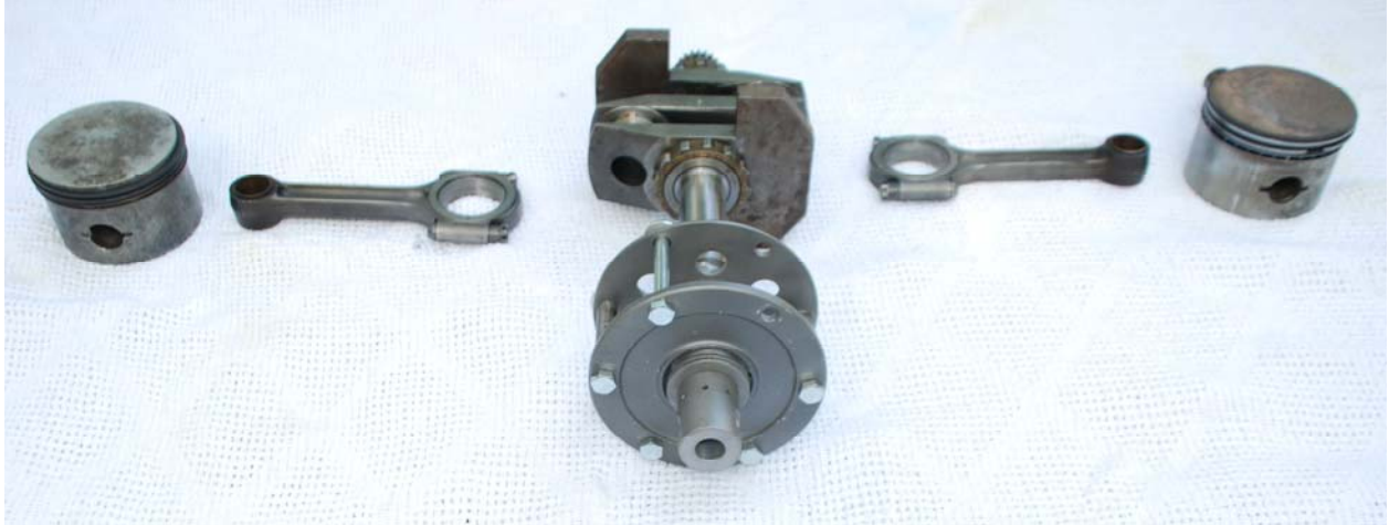
Figure F-1: Aeronca E-113 airplane engine dynamic components including the pistons, connecting rods, and crankshaft shown with the propeller hub mounted
