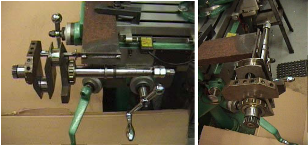
Figure F-4: Fixture for swinging the crankshaft assembly to determine the moment of inertia by supporting on knife edge through the crank pin lightening hole
