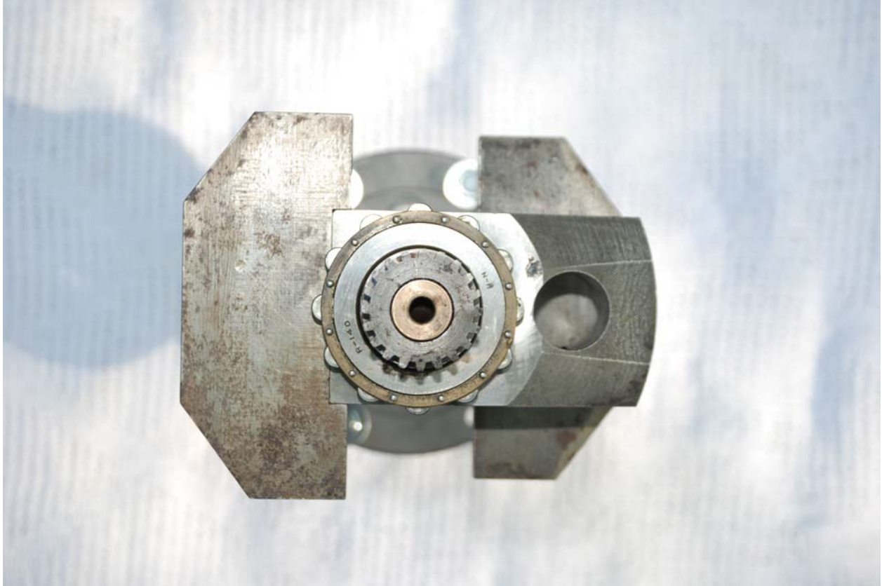
Figure F-3: Back view of crankshaft assembly showing oil spindle hole, timing gear, main bearing, and counterweights
