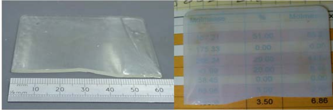
Figure 9 Before annealing ZBLAN glass sample on the left, the same sample after annealing at 290 °C.
