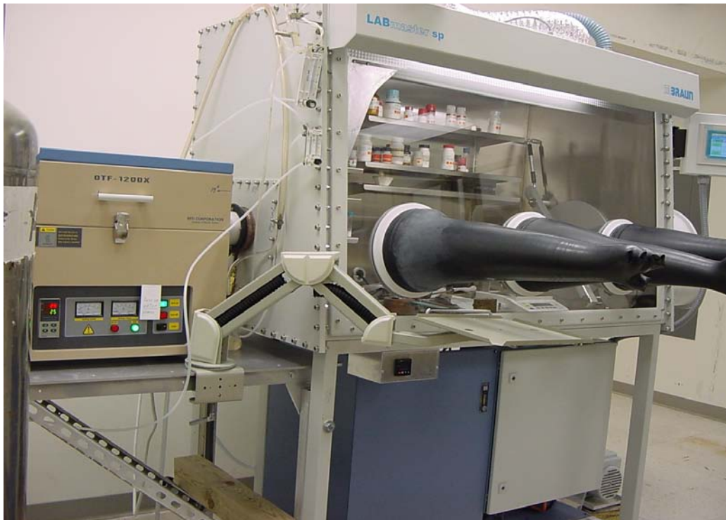
Figure 7 Glove box connected to the furnace on the left
