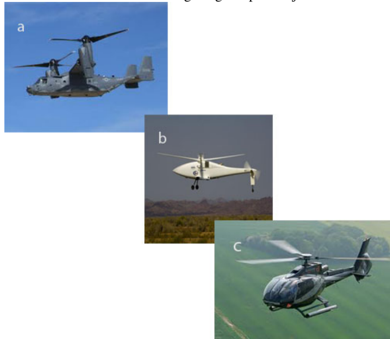
Figure 1.1 Some current rotorcraft employing a variable speed rotor (achieved with engine speed variations); (a) Bell-Boeing V-22, (b) A169 Humming Bird UA, (c) Eurocopter EC130
