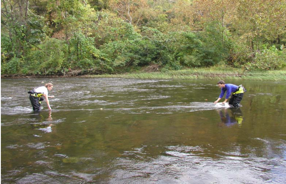
Figure 9. Measuring stream velocity: an orange was timed on a 10-m float downstream. Three velocity measurements were recorded at the site where gilt darters were observed and a mean value determined.
