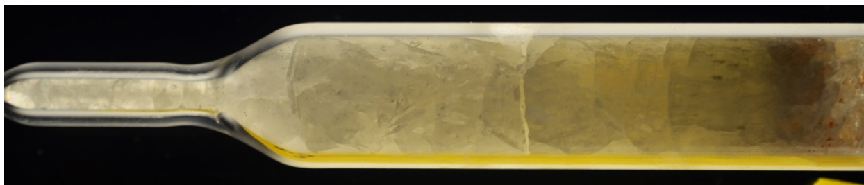
Figure 31. Boule E-68-3 at room temperature after a 48-hour high temperature annealing step exhibiting only minor improvement to the cracking behavior.
