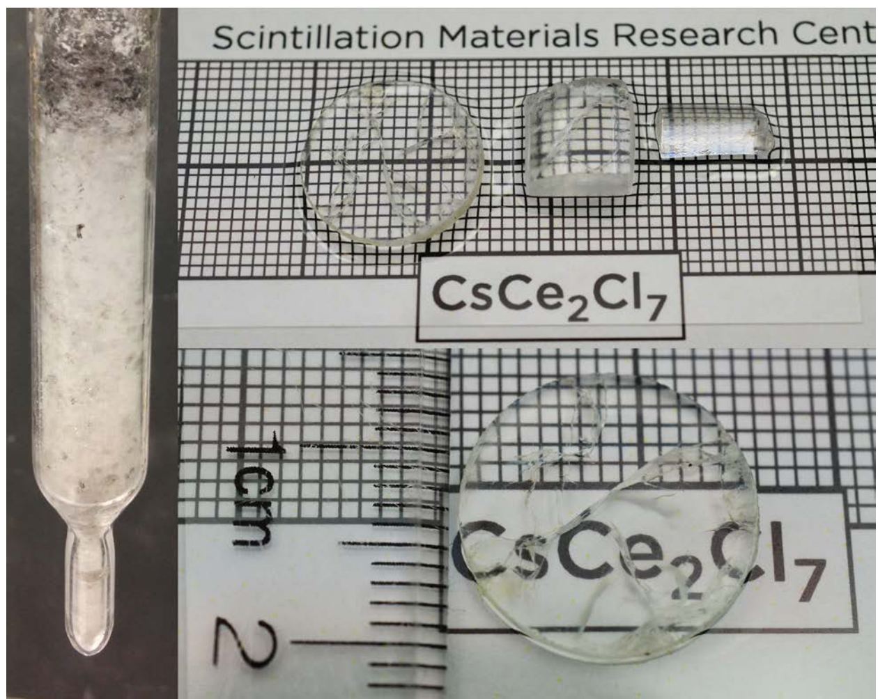
Figure 32. The E-77 boule after growth (left). Portions cut and polished from the boule exhibiting excellent clarity and a reduced cracking behavior with no evidence of visible inclusions.
