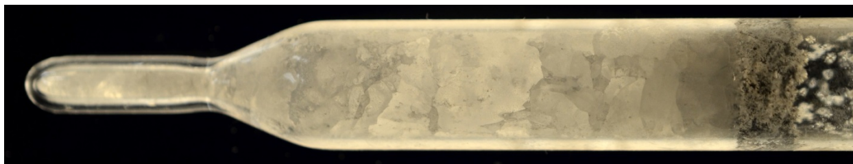
Figure 34. Boule E-82 grown with an argon gas partial pressure over the melt to reduce volatilization. A marked reduction in cracking is observed in a small portion in axial center of the boule. Note the solid condensate in the upper portions of the ampoule indicative of irreversible metal halide volatilization from the melt.
