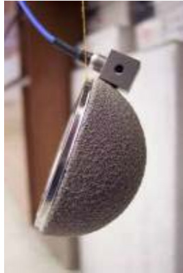
Figure 25. Resonant Test Setup for Acetabular Cup and Liner
