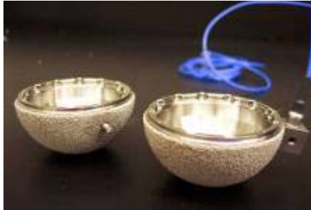
Figure 20. Accelerometer Mount and Mounted Accelerometer on Acetabular Cup
