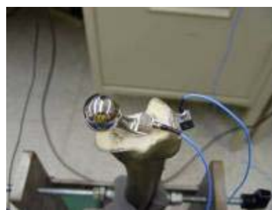
A. Figure 19. A.) Accelerometer Hard Mounted on Back of the Acetabulum B.) Accelerometer Hard Mounted on Greater Trochanter
