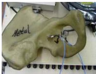
A. Figure 19. A.) Accelerometer Hard Mounted on Back of the Acetabulum B.) Accelerometer Hard Mounted on Greater Trochanter
