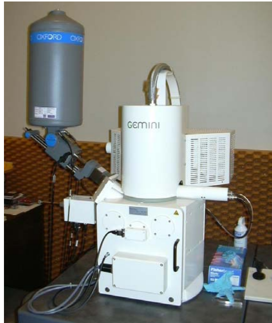
Figure 3.32: Photograph of the scanning electron microscopy hardware with energy dispersive spectrometry detector.
