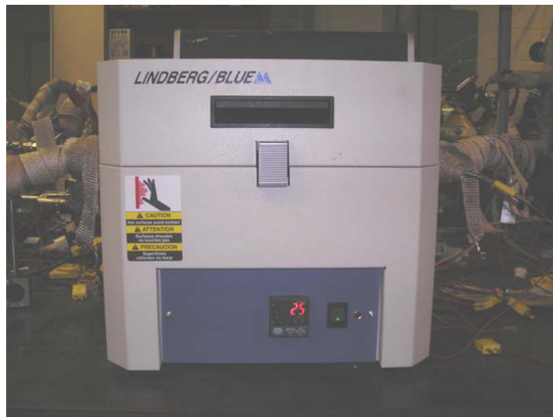
Figure 3.20: Photograph of the Lindberg electric furnace used to maintain the diesel oxidation catalyst operating temperatures.
