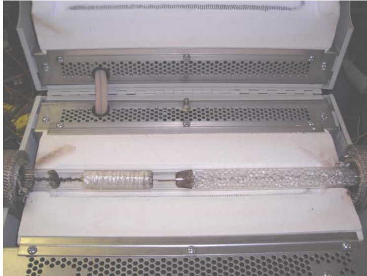
Figure 3.19: Photograph of the DOC reactor placement inside the Lindberg furnace.
