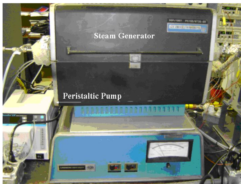
Figure 3.17: Photograph of the steam generator used in the bench-flow reactor system.
