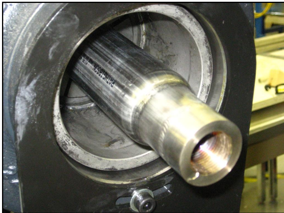
Figure 3.13: Grip sleeve exiting from crimping machine
