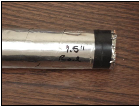
Figure 4.49: Wrap end of cable with tape to prevent foil from unwrapping
