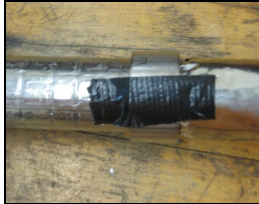
Figure 4.58: Grip ring taped in place in preparation for swaging
