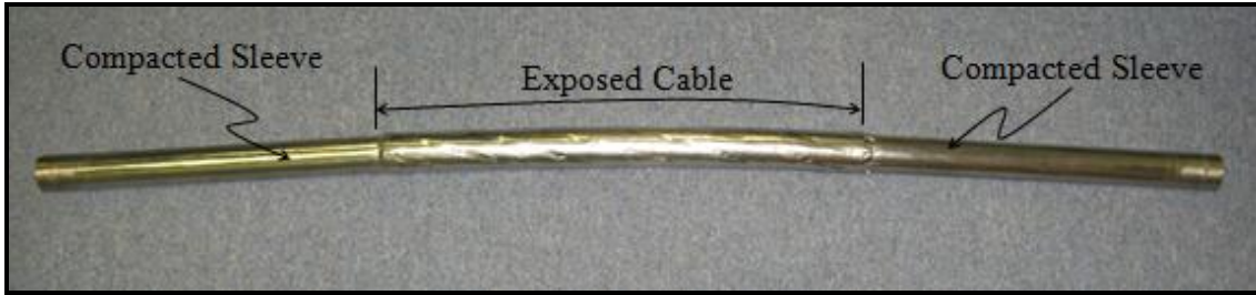
Figure 3.14: Fully assembled full scale TF pull test sample
