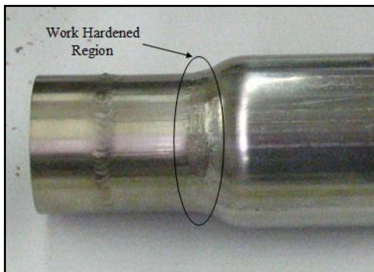
Figure 3.15: Work hardened region on pre-crimped sleeve
