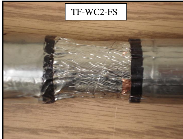
Figure 4.68: Grip sleeve failure due to sleeve slippage
