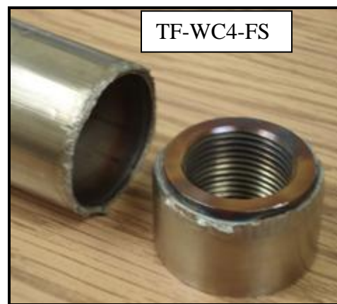
Figure 4.70: Grip sleeve failure due to seam weld fracture
