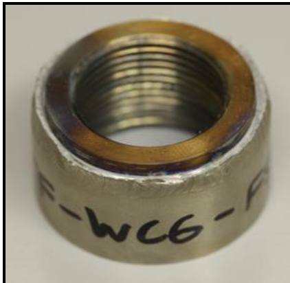
Figure 4.102: TF-WC6-FS seam weld fracture
