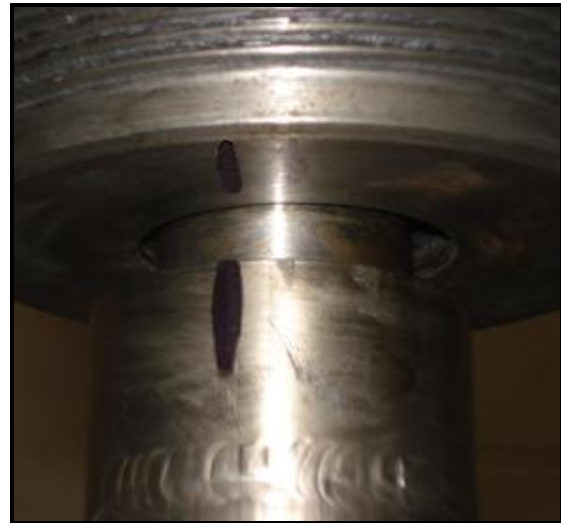
Figure 4.65: Reference lines to monitor specimen rotation
