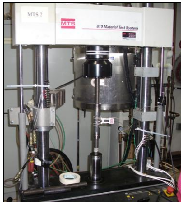
Figure 4.1: Equipment Setup for Preliminary Pull Tests
