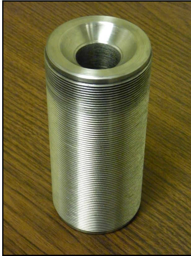
Figure 4.19: Main anchor component for upper dynamic coupling
