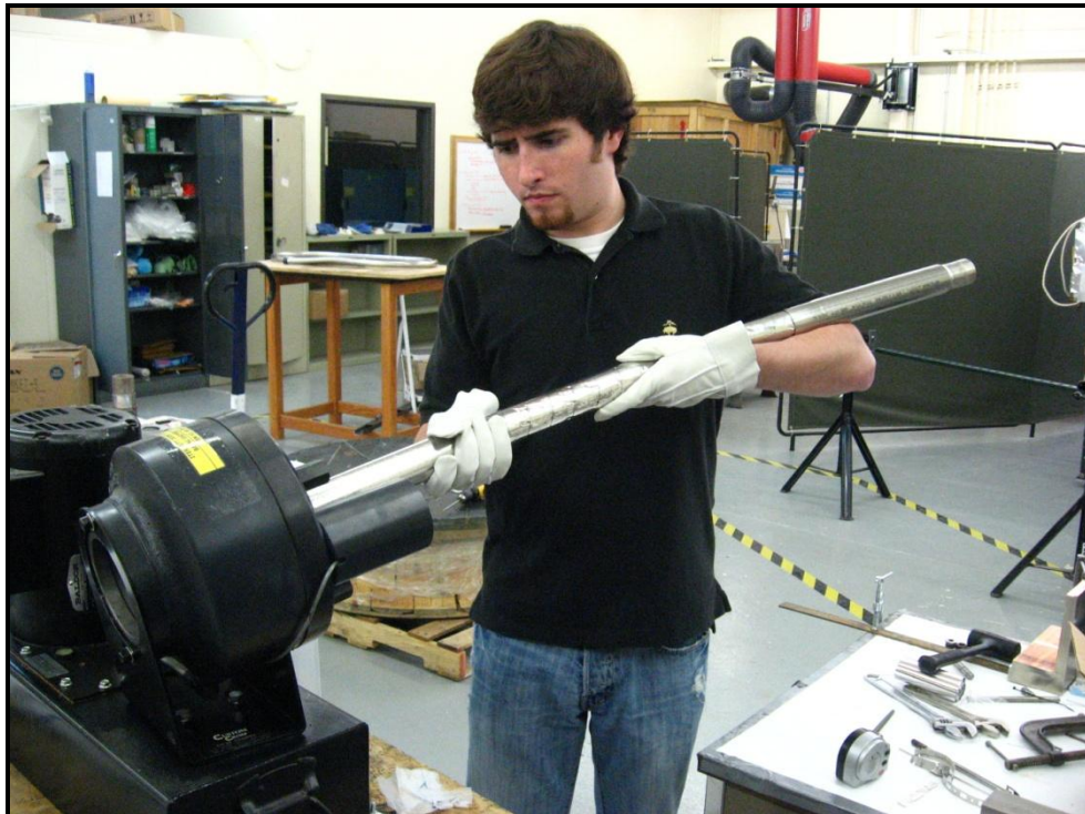
Figure 3.11: Initial stages of TF grip sleeve compaction
