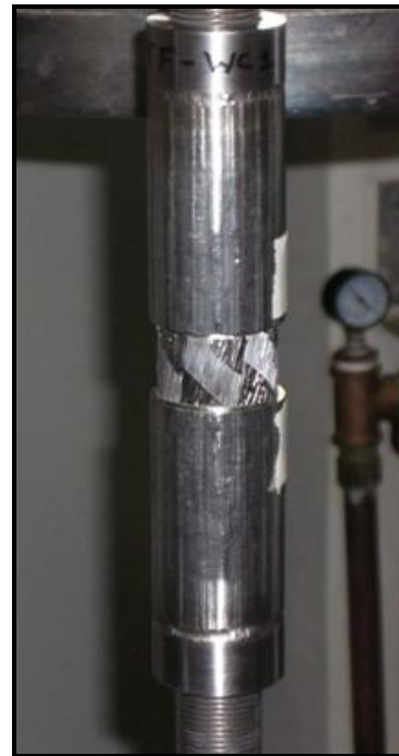
Figure 4.9: TF-WC1 grip sleeve position after testing
