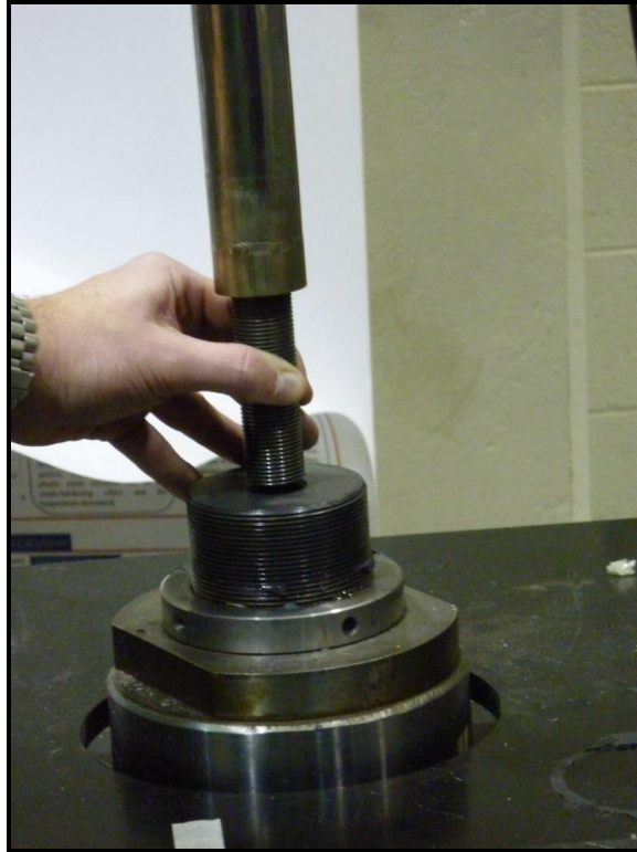
Figure 4.29: All-thread rod contacting lower coupling
