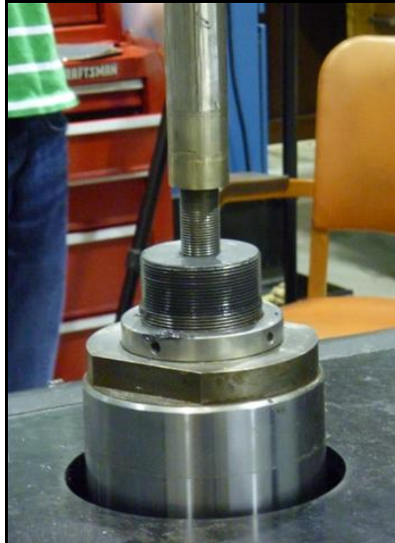
Figure 4.30: Test specimen mounted to fixture's hydraulic actuator
