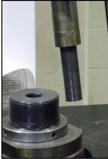
Figure 4.28: All-thread rod installed in lower tensile lug
