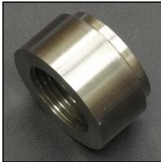
Figure 3.17: Side view of threaded tensile lug
