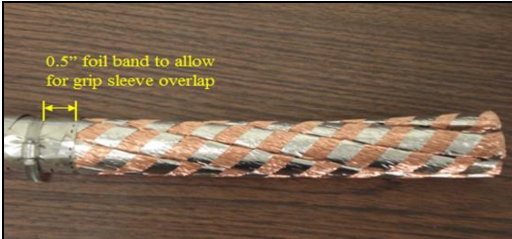
Figure 4.53: End of cable with foil removed showing 0.5" foil band for grip sleeve overlap
