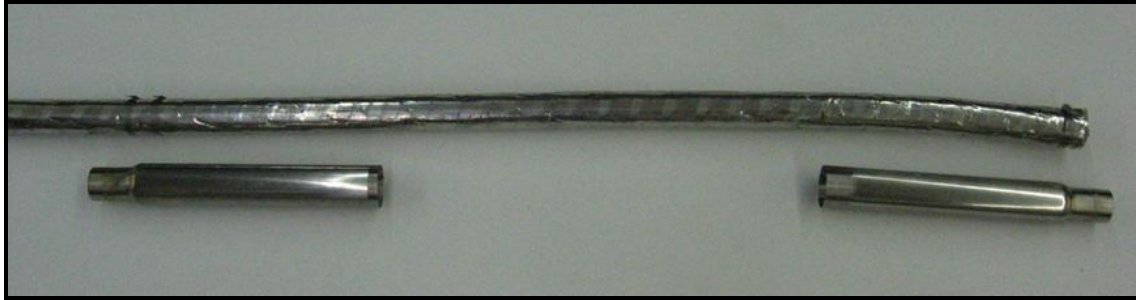
Figure 3.6: Pre-crimped grip sleeve compared to nominal cable diameter
