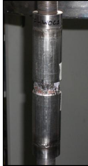
Figure 4.11: TF-WOC1 grip sleeve position after testing
