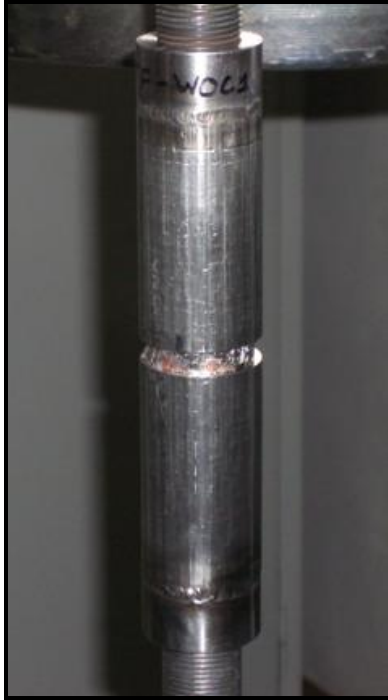
Figure 4.10: TF-WOC1 grip sleeve position before testing
