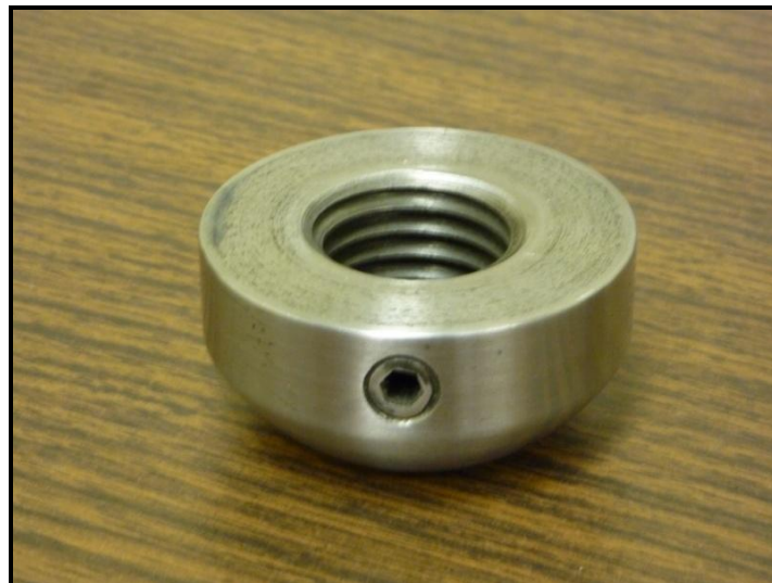
Figure 4.20: Hemispherical nut for upper sample support
