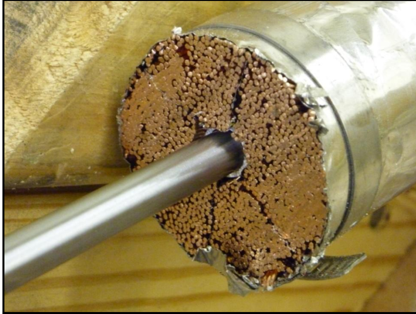
Figure 3.8: Insertion of solid rod into core tube of TF cable
