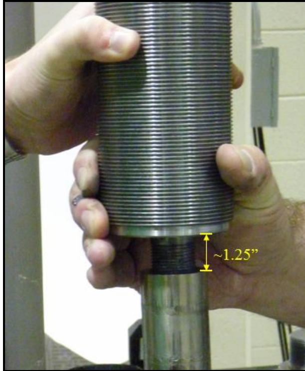
Figure 4.26: Dynamic coupling connected to upper tensile lug
