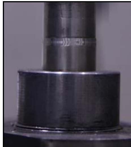
Figure 4.76: Lower tensile lug tightened flush with coupling to prevent rotation
