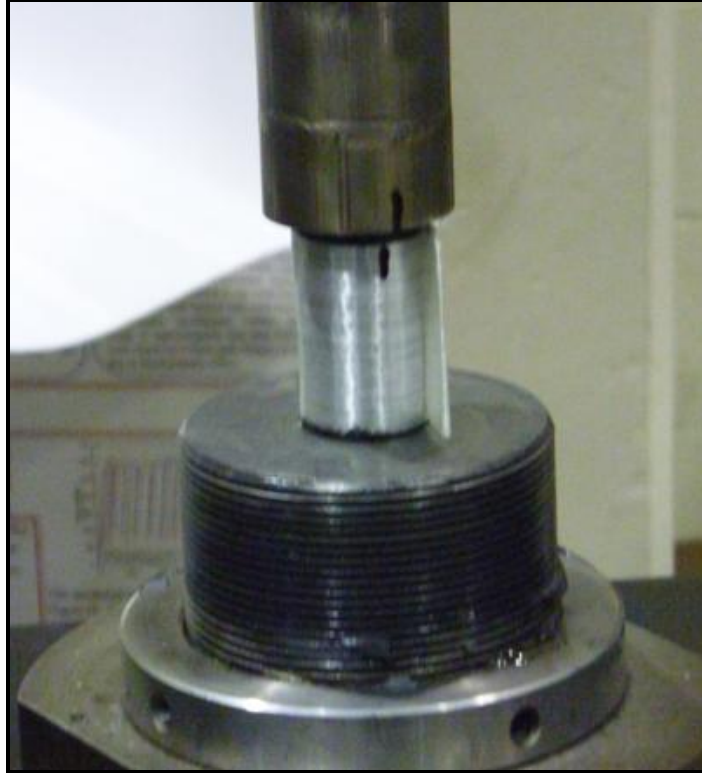
Figure 4.32: Vertical markings to monitor displacement due to rotation
