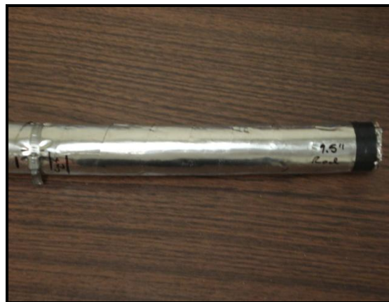
Figure 4.51: Reference lines marked to indicate where to cut foil
