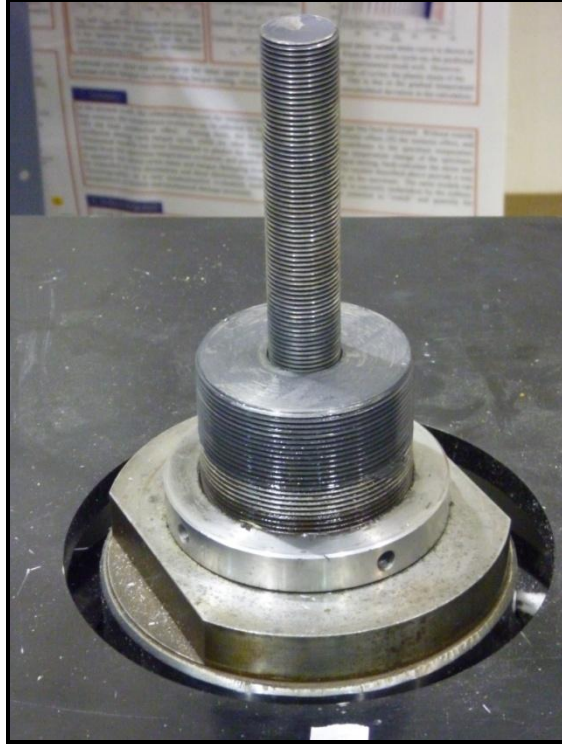
Figure 4.18: Fully assembled static coupling mounted to hydraulic actuator
