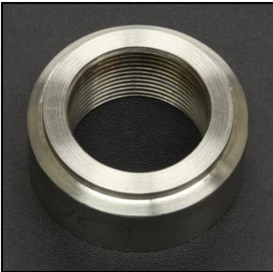
Figure 3.16: Bottom view of threaded tensile lug
