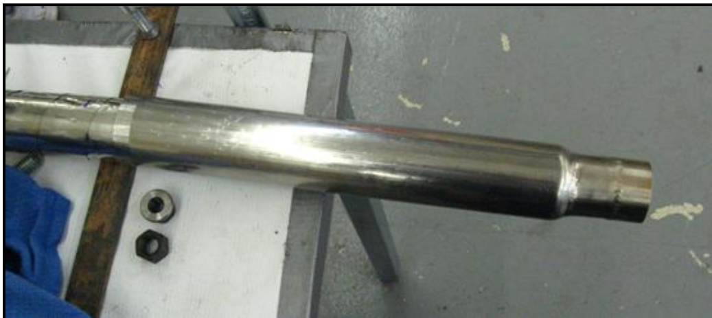
Figure 3.9: Grip sleeve positioned on TF cable prior to compaction
