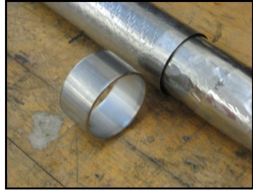
Figure 4.56: Uncompacted grip ring compared to partially compacted sleeve
