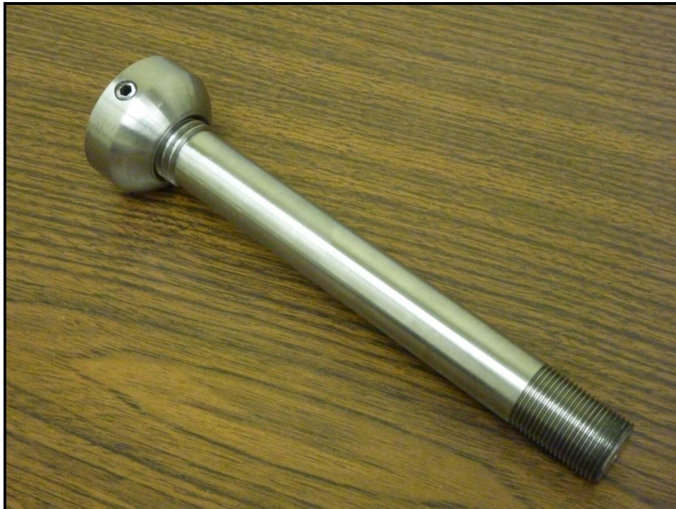
Figure 4.22: Assembled upper sample attachment rod
