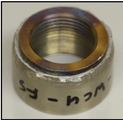
Figure 4.100: TF-WC4-FS seam weld fracture
