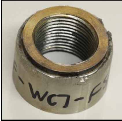
Figure 4.104: TF-WC7-FS seam weld fracture
