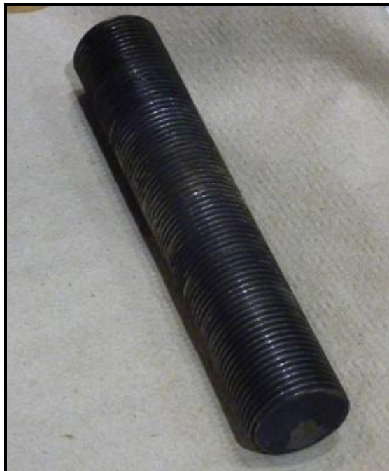
Figure 4.17: All-thread rod to mate test sample and fixture
