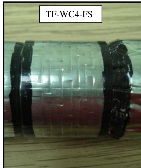
Figure 4.63: Double accent band for samples with reinforcement grip ring
