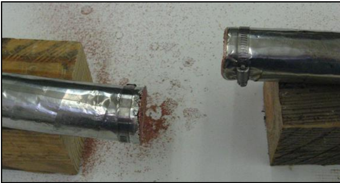
Figure 3.7: Hose clamps positioned around cut to prevent unwinding
