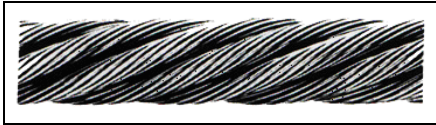
Figure 2.1: Wire rope featuring Left hand Lay strand orientation [26]
