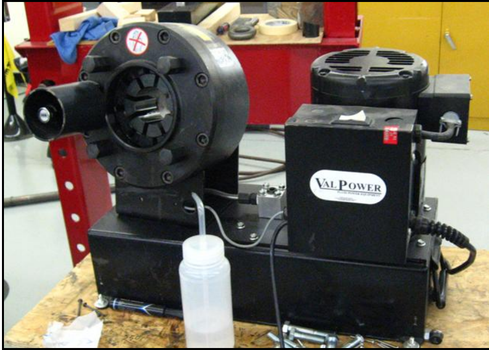
Figure 3.10: Val Power material crimping machine used during test sample fabrication
