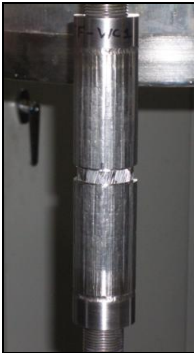
Figure 4.8: TF-WC1 grip sleeve position before testing
