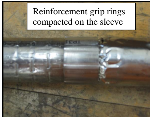
Figure 4.59: Reinforcement grip ring after compaction around grip sleeve
