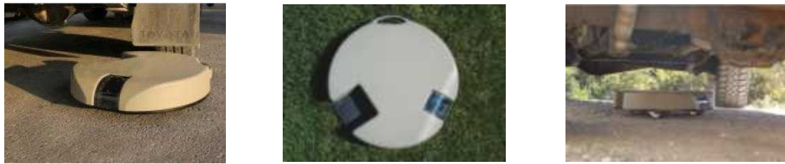
(a) Specter Omni-Directional Under vehicle Inspection System by Autonomous Solutions Inc. [36].
