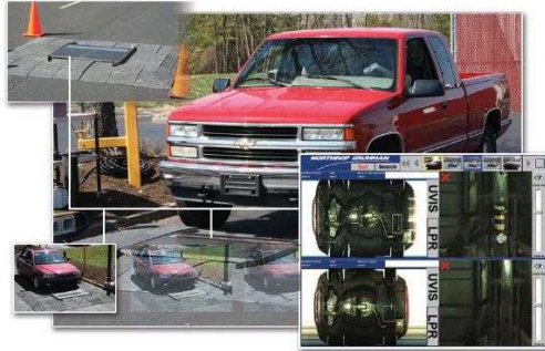
(a) Under vehicle inspection system by Northrop Grumman [42].
