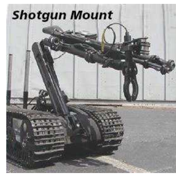
Figure 14: Different application specific designs of the TALON family of robots manufactured by Foster Miller Inc. [34].
