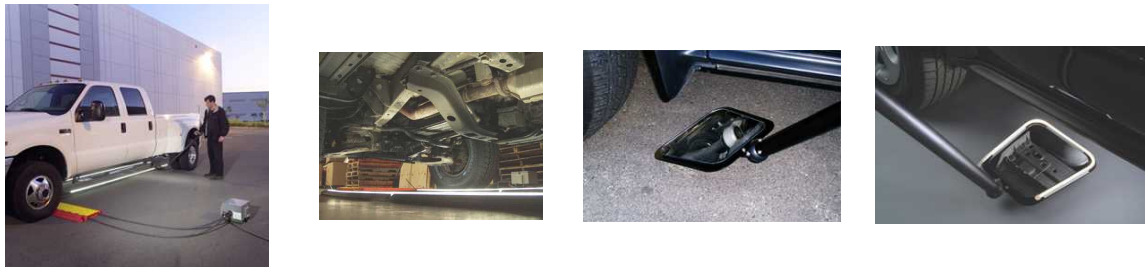
(c) Under vehicle inspection systems by Lumenyte International Corporation [41].
