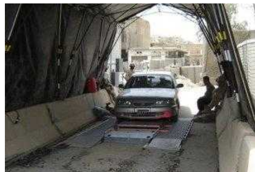
(f) Under vehicle inspection system by Gatekeeper Inc. [47].
