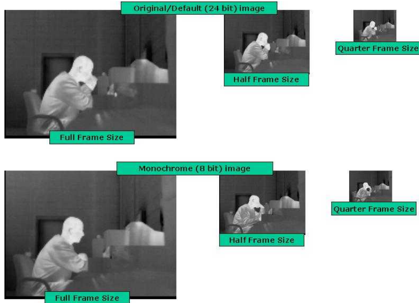
Figure 26: Top row shows different frame sizes of the original or default data type (24-bit image). Bottom row shows different frame sizes of the monochrome data (8-bit image).
