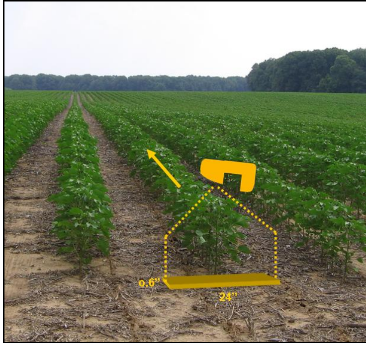
Figure 12. GreenSeeker® sensor followed rows direction when collecting data. Field of view for each measurement from the GreenSeeker® sensor is approximately 24x 0.6 inches.
