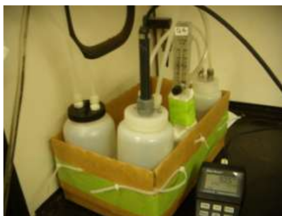
Figure 2.12 Aging with 90% RH in ambient temperature: Schematic of aging system (up) and experiment setup (down).
