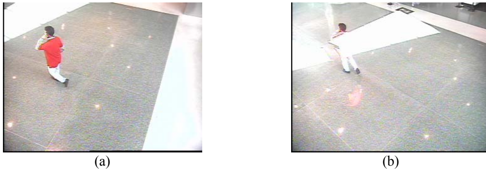
Figure 1.3 Two consecutive frames of a scene illustrating the effect of illumination on the color image formation.
