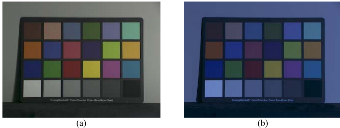
Figure 1.1 Macbeth color checker under different illuminant. (a) Phillips Ultralume fluorescent tube (b) Solux 3500K +Roscolux 3202 blue filter [Barnard'02c].
