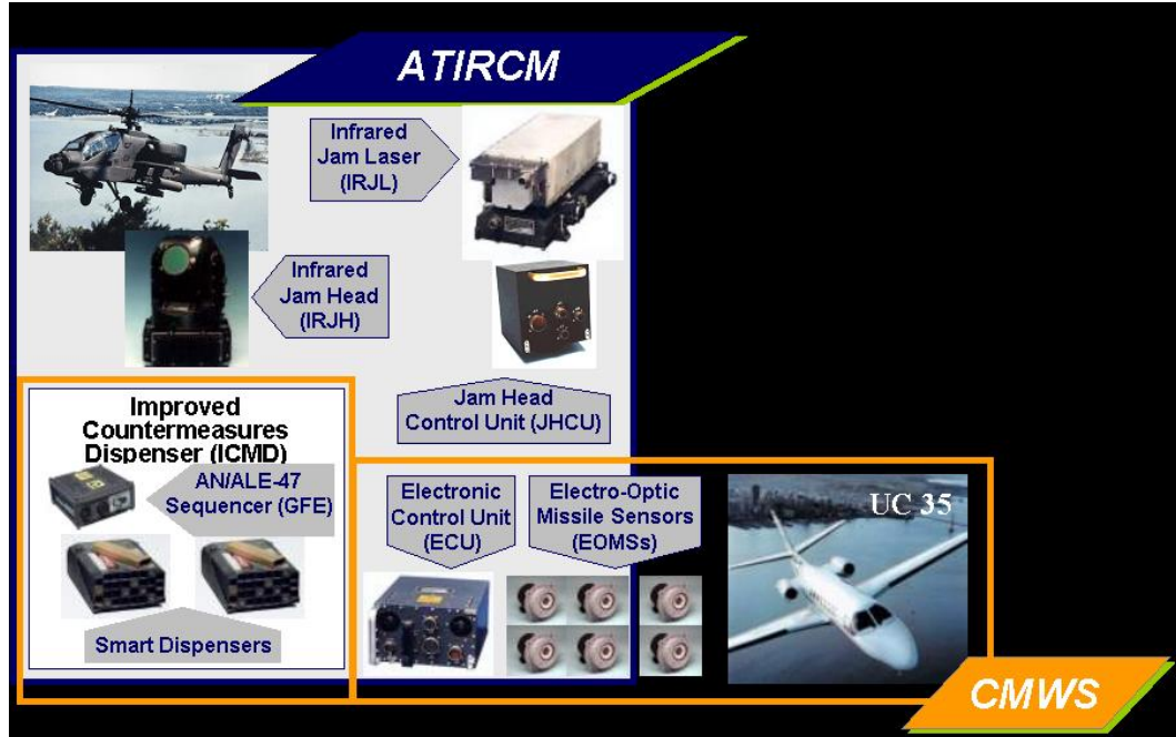
Figure 3-1. Army ATIRCM/CMWS Components Source: PM, AES, ATIRCM/CMWS Brief, August 2004
