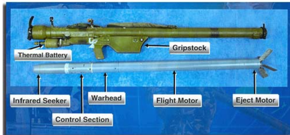
This image identifies the main components of a typical MANPADS.
