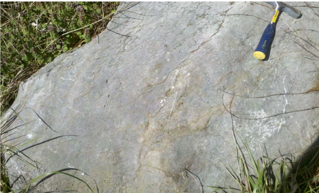
Figure 2-24. Exposures of Lenoir Limestone showing (A) wavy-bedded to fine-nodular limestone with several 0.5-2 cm thick clay seams located northwest of the Poplar Springs Road/Bright Hope Road intersection, and (B) the Mosheim Member consisting of massive fine-grained limestone near the Pulaski fault contact along Bright Hope Road. (Hammer is ~30 cm long).
