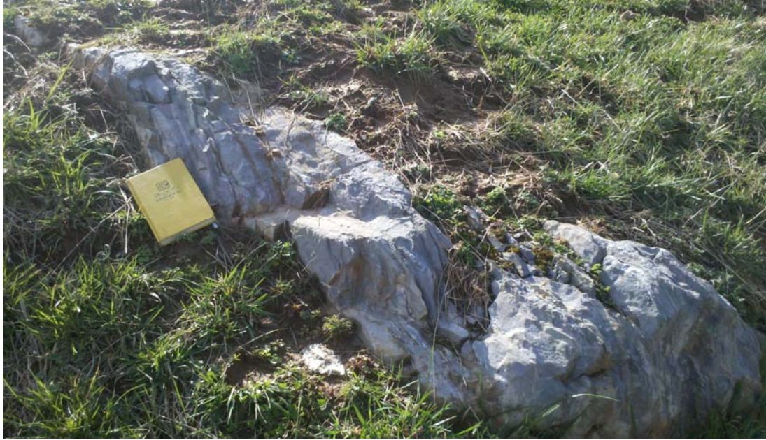
Figure 2-22. Exposure of Kingsport Formation showing bluish-gray fine-grained limestone with thinly ribboned (0.5-1 cm) dolomite. Location is east of Bethel Church near the Pulaski fault trace. (Field book is ~12 x 19 cm).
