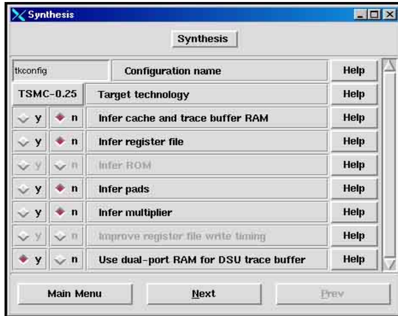
Figure 4.3.2 LEON-2 processor: Synthesis customization
