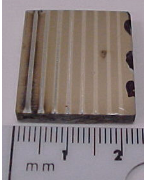
Figure 40 : A finished Cr substrate sample with eight combinatorial EB welds across the length of the wedged Ni film.
