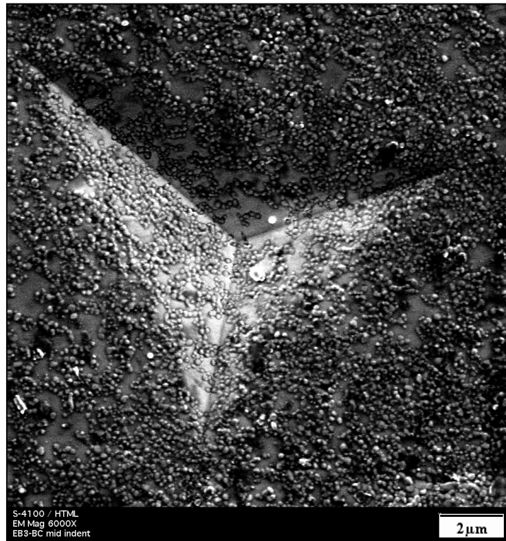
Figure 10 : SEM image of typical indent made in the EB weld surface.
