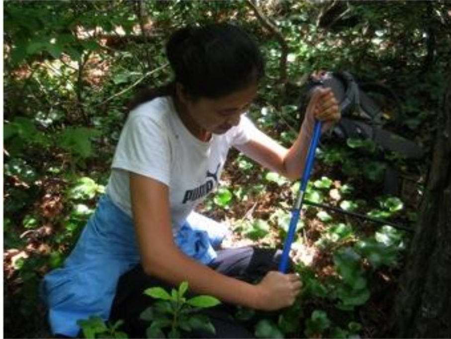
Figure 5. A core being extracted from the base of a Table Mountain pine on Linville Mountain. (Photo © H.D. Grissino-Mayer)
