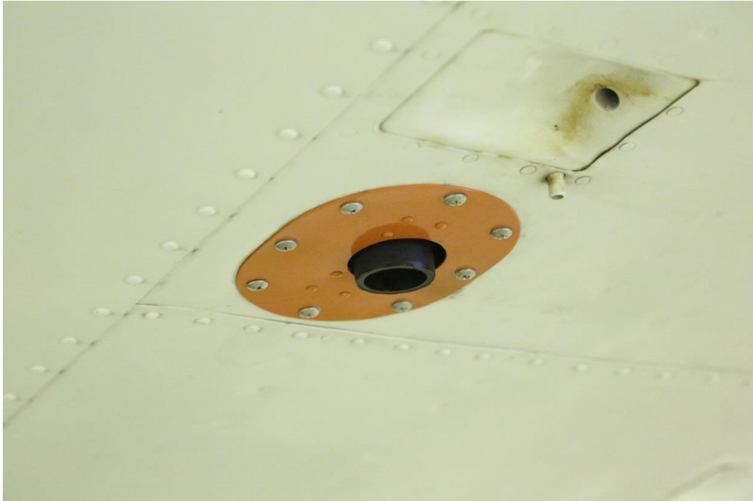
Figure 9b: The Axis 221 camera mounted under the left wing of the Navajo (close up).
