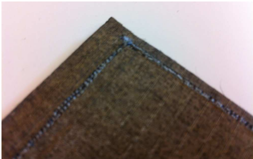
Figure 79: Conductive vias implemented with two rows of closely stitched conductive thread.
