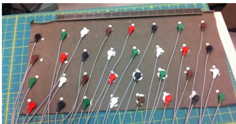
Figure 38: Large conductive textile sample with electrodes connected.
