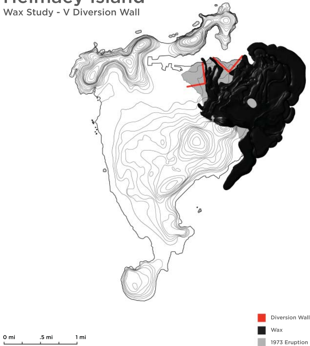
Figure 5.01 Wax Study - V Diversion Wall Source: Author; Map Based off of: ArcGIS
