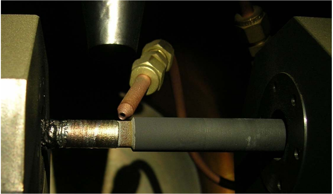
Figure 4.3.1(a) A 20 mm long molybdenum cylinder made on a molybdenum coated graphite mandrel.
