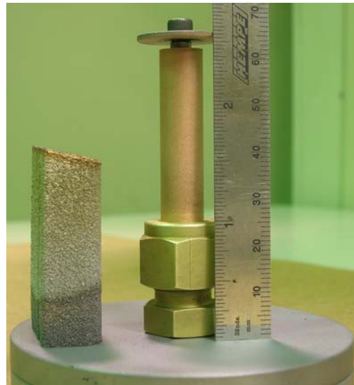
Figure 10 – A 40 mm AISI H13 steel solid freeform fabricated extrusion of the University of Tennessee logo.
