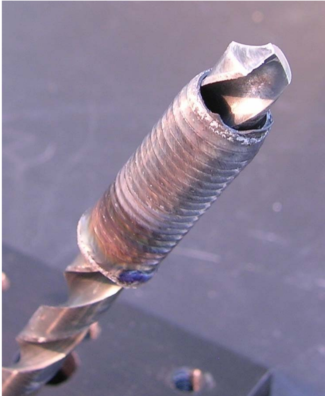
Figure 4.3.3(d) A 30 mm long and 1 mm thick W-TiC cylindrical deposit made on a graphite mandrel by laser processing a 1.3 mm thick W-TiC barrier coating at 1600 W.
