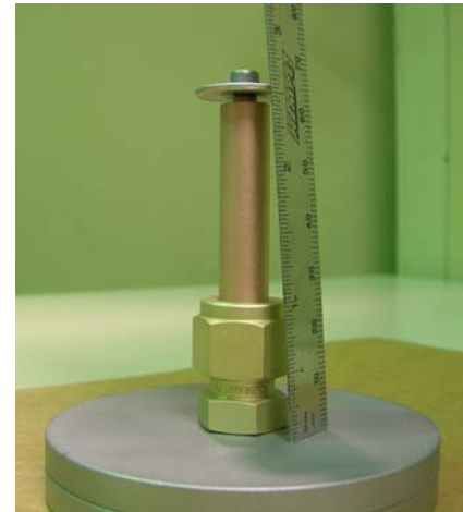
Figure 4 – A 2 ½” tall prototype tower nozzle in service at UTSL.
