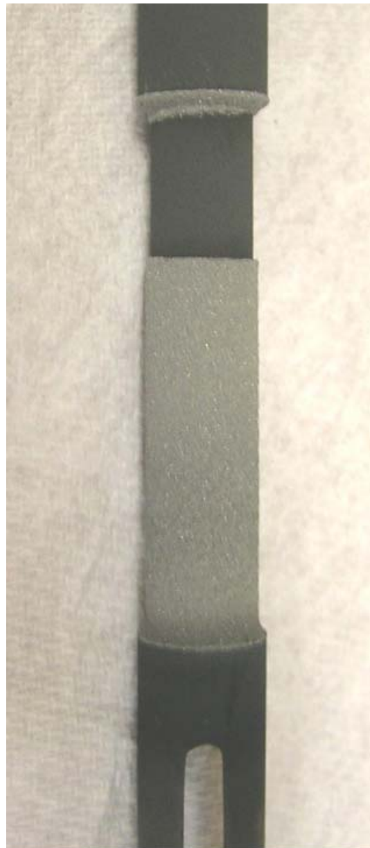
Figure 3.8. An induction hardened barrier coating on a graphite mandrel.
