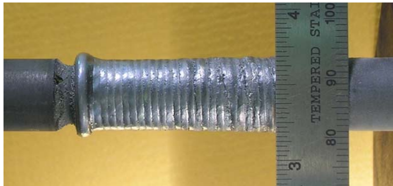
Figure 17 – A 30 mm long cylinder produced using a \frac{3}{4} (32-38 \mu\text{m} W) + \frac{1}{4} (75-106 \mu\text{m} APS W-coated TiC) powder mix.
