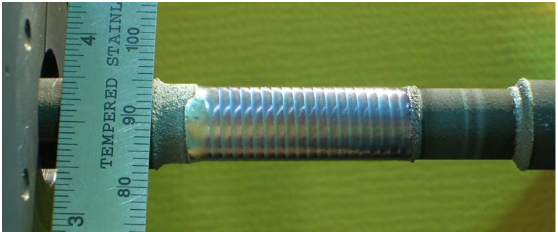
Figure 4.3.3(a) A 30 mm long and 0.3 mm thick W-TiC deposit made on a graphite mandrel by laser processing a 0.6 mm W-TiC barrier coating induction hardened for 5 hours. Laser processing was done at 1500 W.
