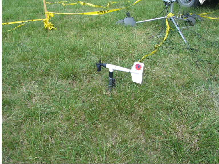
Figure 1.5: The Young's wind monitor measures vector averaged windspeed.
