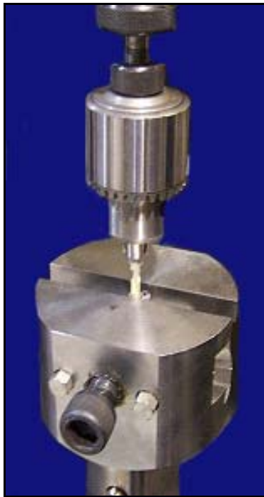
Figure 3.8. Tensile test with specimen held by clamps
