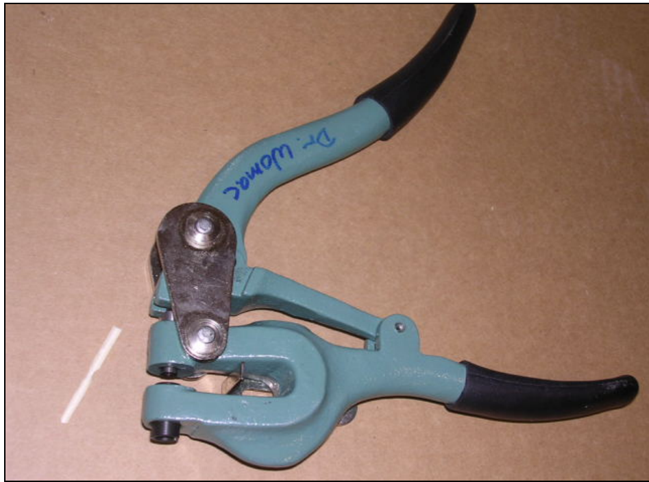
Figure 3.10 A circular hole puncher for cutting switchgrass sample notch
