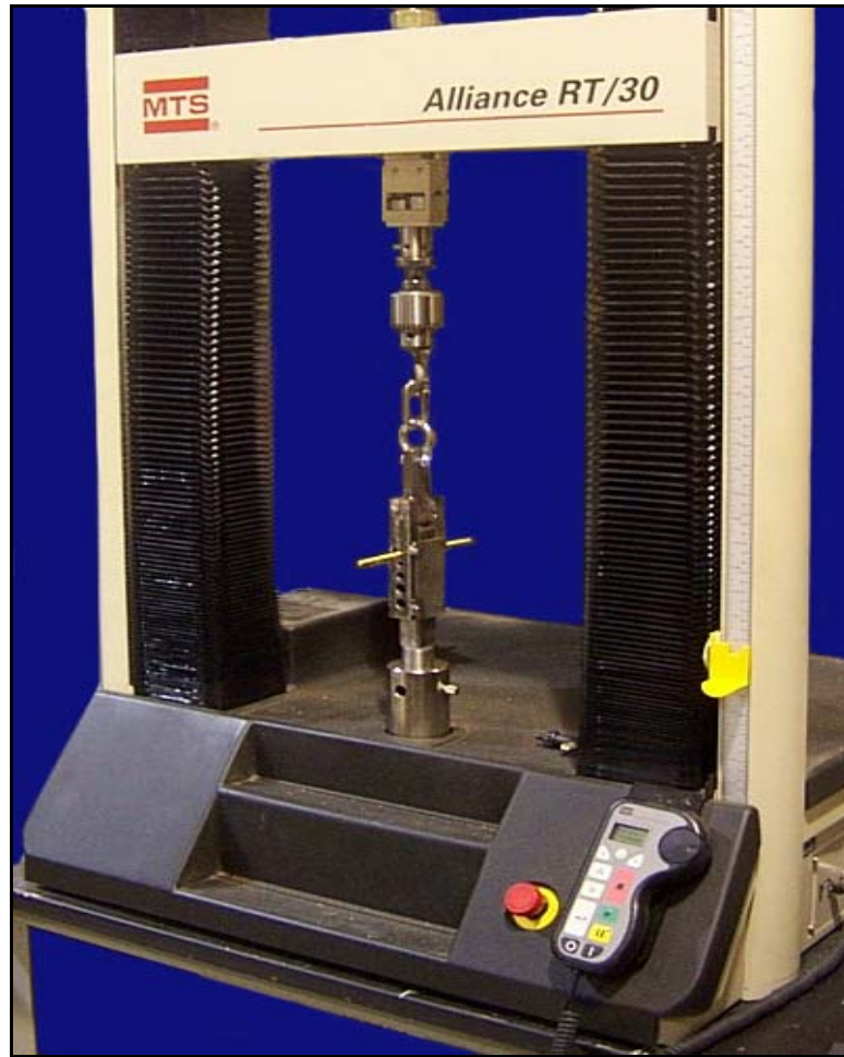
Figure 3.6. Universal testing machine (mounted with tools for shear test)
