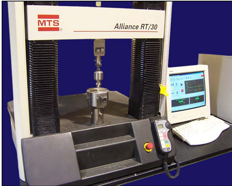
Figure 3.5. Universal testing machine (mounted with tools for tensile test)
