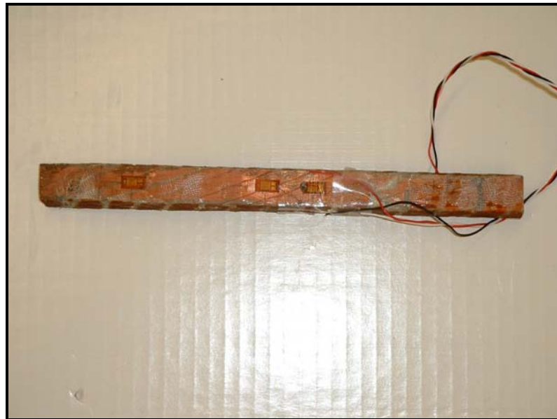
Fig: 6.3 Copper-CTD-101K composite bar with strain gages.
