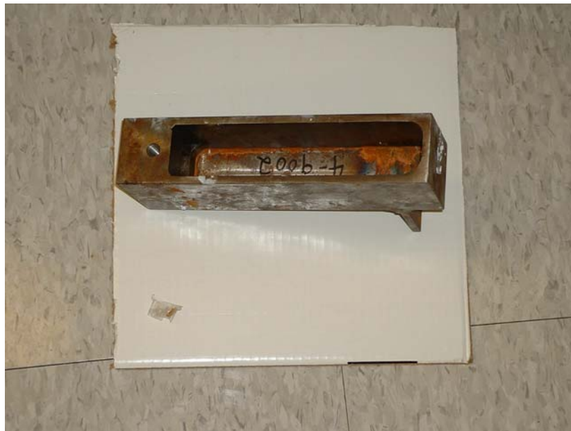
Fig 6.4: Fixture for cantilever beam bend test.
