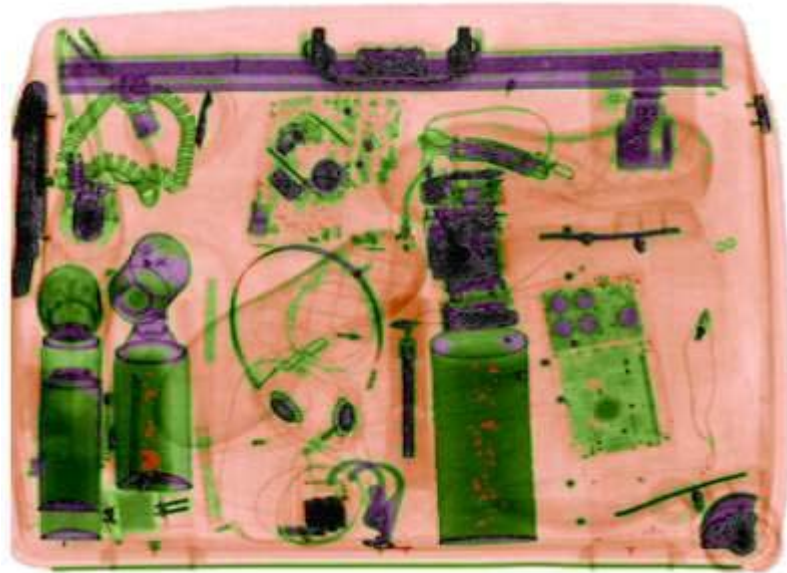
Figure 5: An X-ray of a bag. Notice that all organic items are a shade of orange 37
