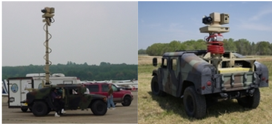
Figure 20: Viper system mounted on a HUMMUV with telescopic arm
