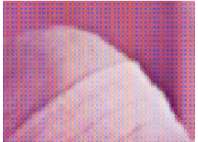
(d) Zoomed version of the demosaicked output showing the zipper effect
