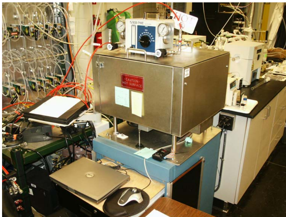
Figure 3.10. Spatially-Resolved Capillary Inlet Mass Spectrometer
