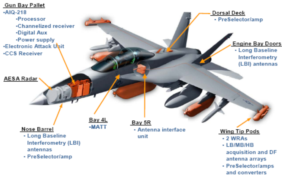
FIGURE 3: E/A-18G AIRBORNE ELECTRONIC ATTACK SUITE
