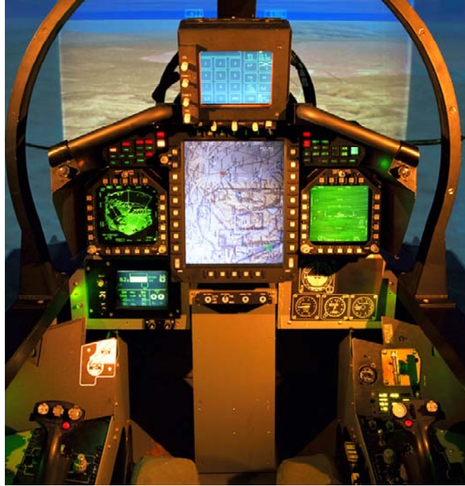
FIGURE 7: E/A-18G AFT COCKPIT
