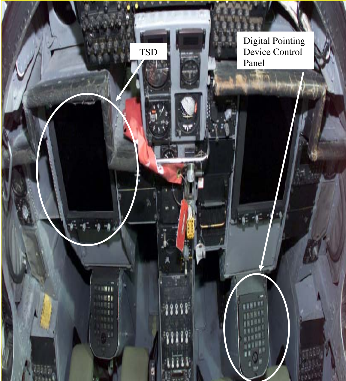
FIGURE 5: ECMO 2 AND 3 DISPLAYS AND CONTROLS
