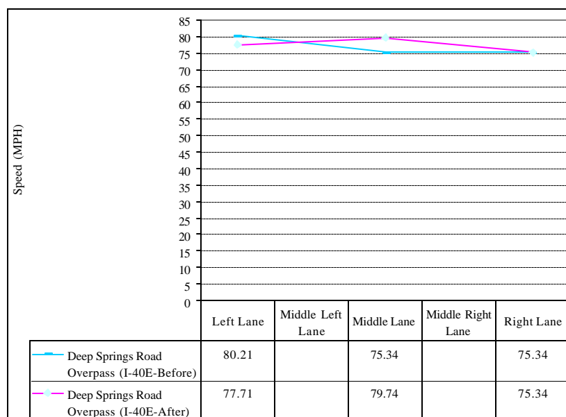
Figure 7-04. Truck speed in westbound direction at Deep Springs road overpass in midday time period
