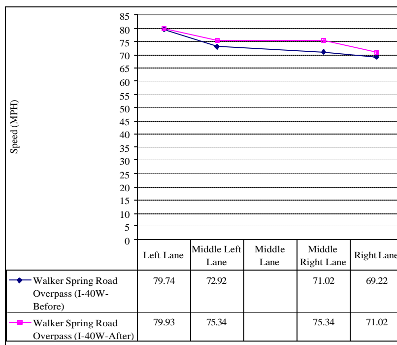
Figure 7-14. Truck speeds in westbound direction at Walker Spring road overpass in the morning time period
