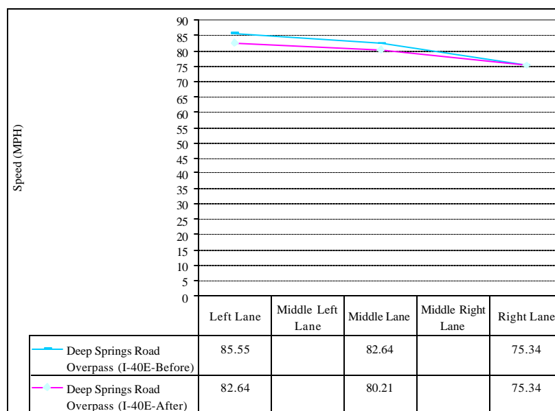
Figure 7-06. Truck speed in westbound direction at Deep Springs road overpass in evening time period
