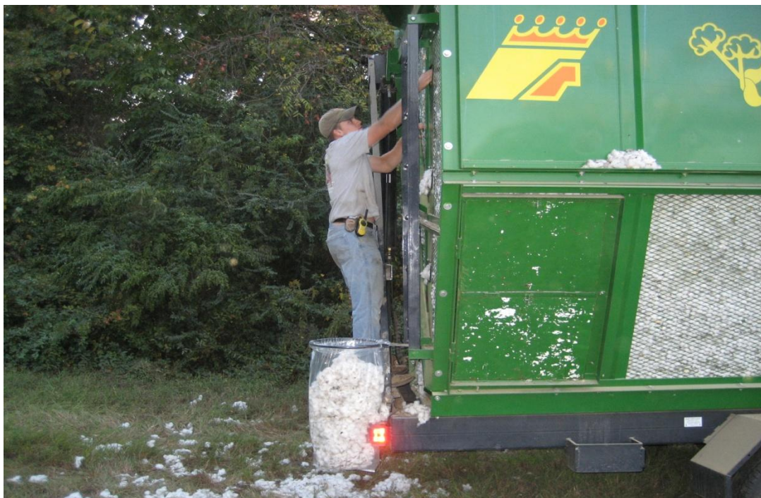
Figure 3. Composite sample are collected from multiple sampling points throughout the boll buggy.
