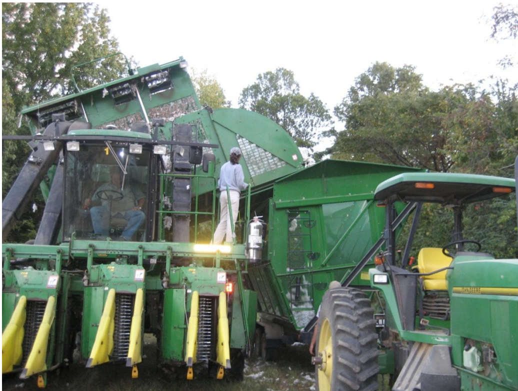
Figure 2. Cotton being unloaded from picker basket to boll buggy to obtain weight and to collect samples.
