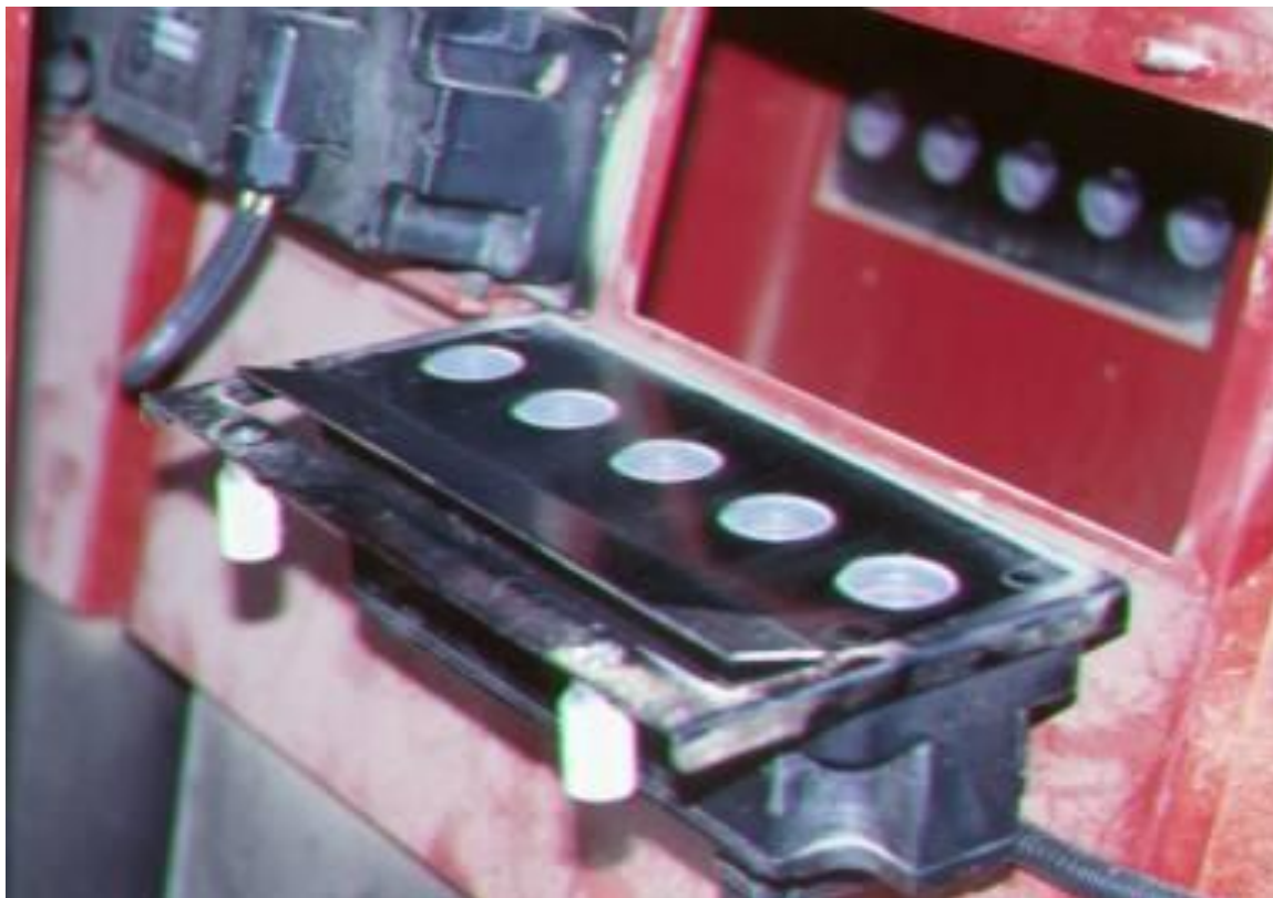
Figure 1. Dust accumulation was cleaned from the sensors at the beginning of the harvest season.
