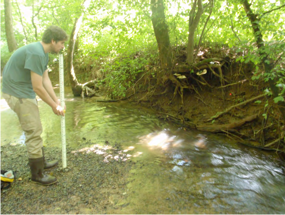
Figure 3.2 Profiling technique with laser point visible on bank of Nails Creek. Photo by Monica Rother.
