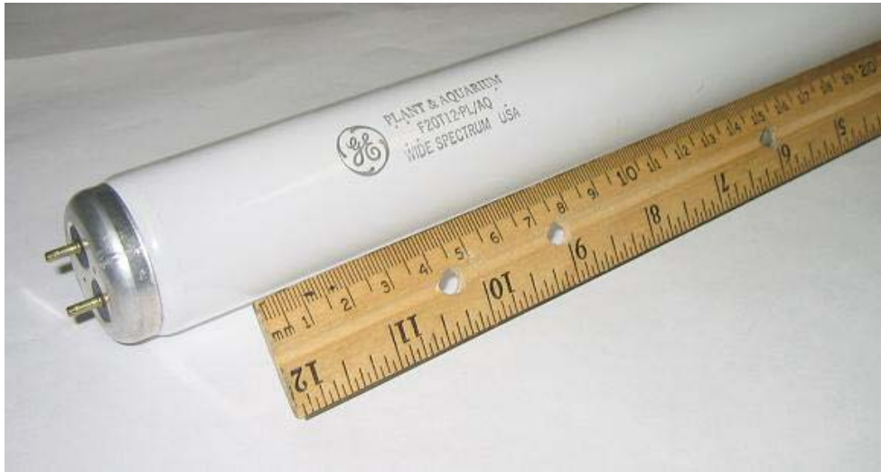
Figure 4.1.1: Mercury-based fluorescent lamp.
