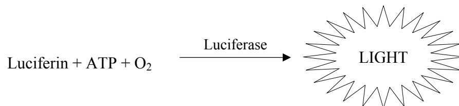
Figure 2.1: ATP Bioluminescence Reaction
