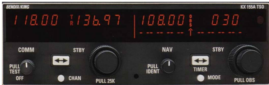
Figure A-13 Bendix/King KX 155A NAV/COMM
