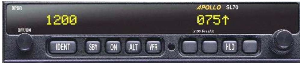
Figure A-14 Apollo SL70 Transponder
