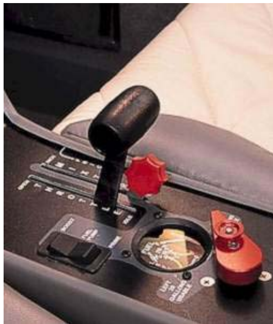
Figure A-24 Cirrus SR20 Center-Mounted Throttle
