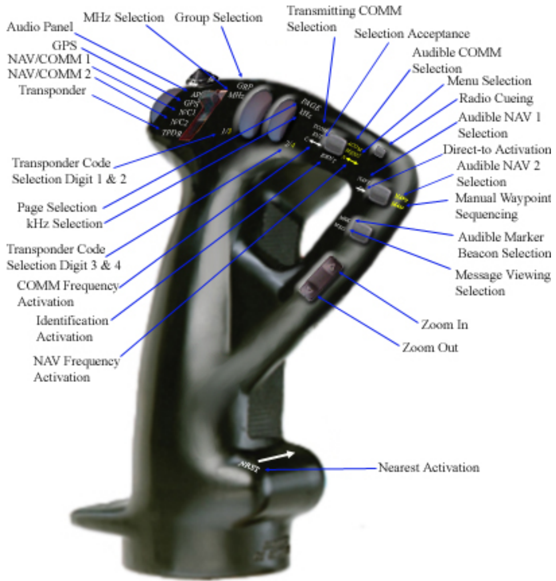
Figure A-49 HOTAS Control Grip with Labels
