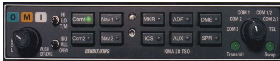
Figure A-7 Bendix/King KMA 28 Audio Panel
