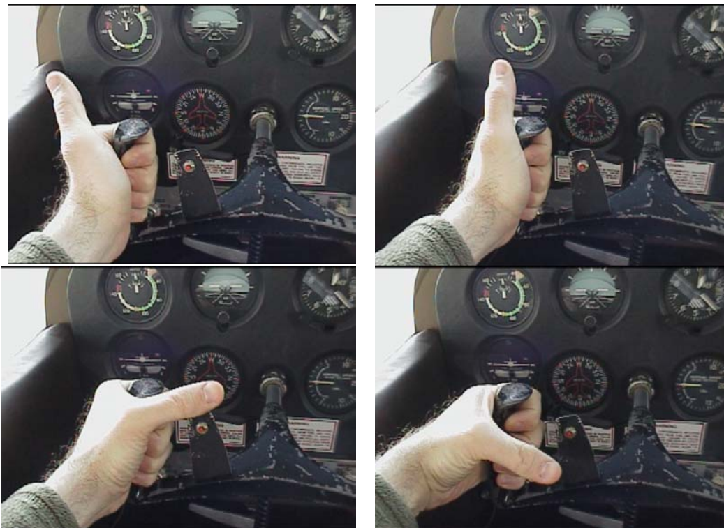
Figure A-45 Thumb Range of Motion Arc about the Control Wheel Grip
