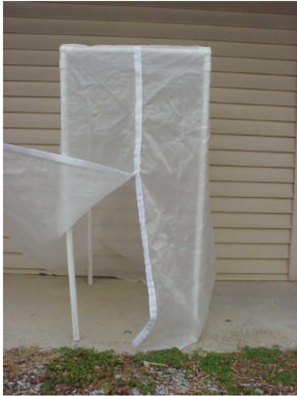
Figure 4.1. Cages constructed of PVC pipe and thrips screen for use in greenhouse experiment.
