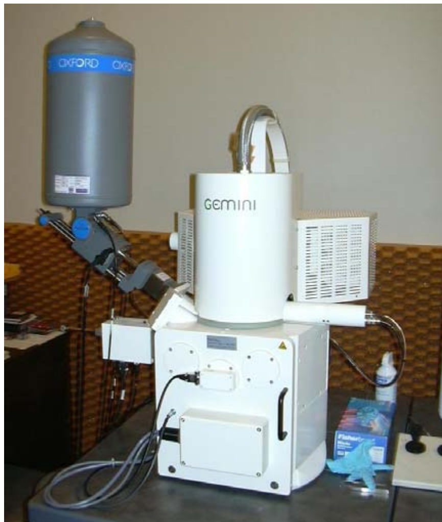
Figure 3-22. Scanning electron microscope with energy dispersive spectrometry detector
