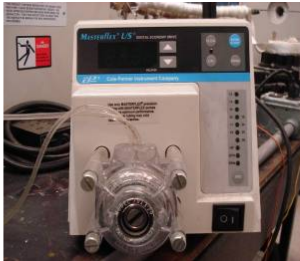
Figure 3-4. Peristaltic pump used to inject de-ionized water into steam generator
