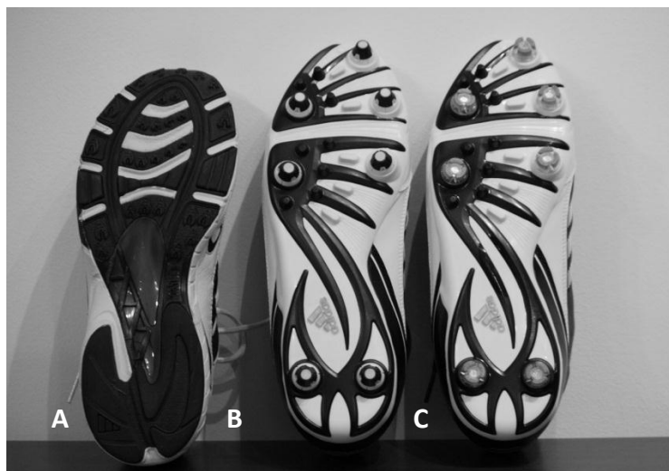
Figure 16: Testing shoes used in the study: running shoe (A, Shoe), football shoe with removable natural turf studs (B, Natural turf cleat) and, football shoe with removable synthetic turf studs (C, Synthetic turf cleat)
