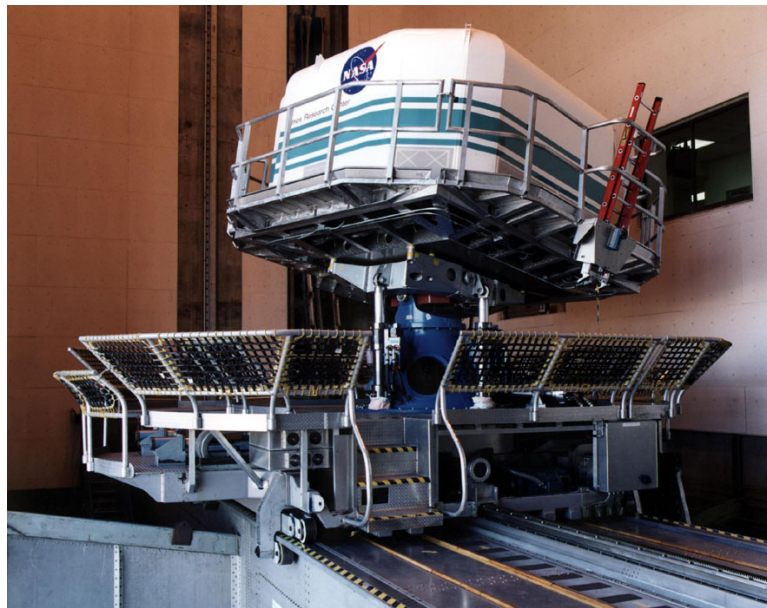
Figure 4. NASA Ames Vertical Motion Simulator Cab and Track
