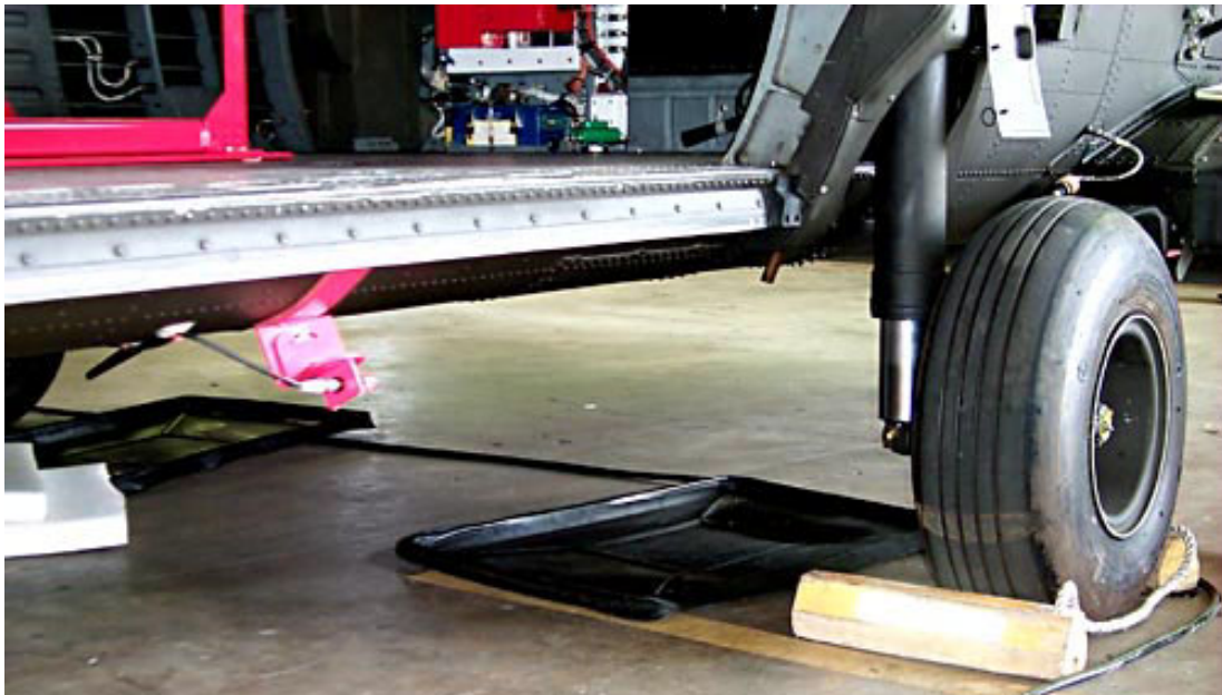
Figure A-4. Main Landing Gear Camera Position (same both sides)
