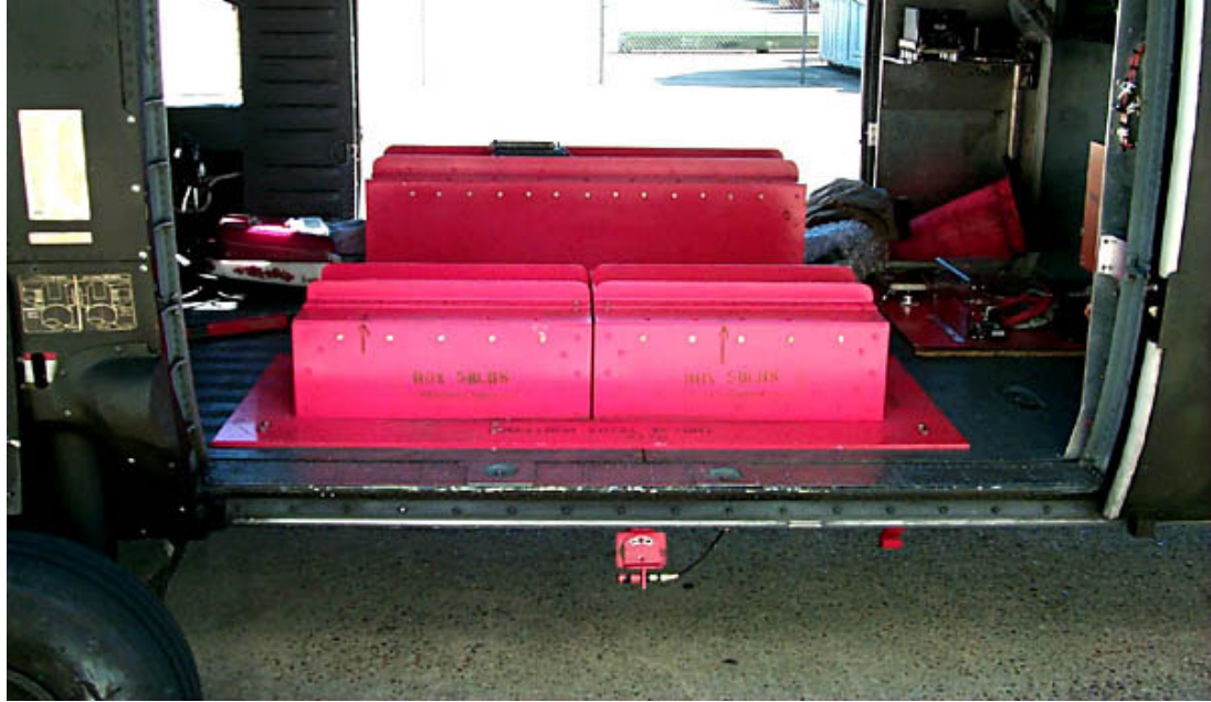
Figure A-3. Main Cabin Ballast Boxes
